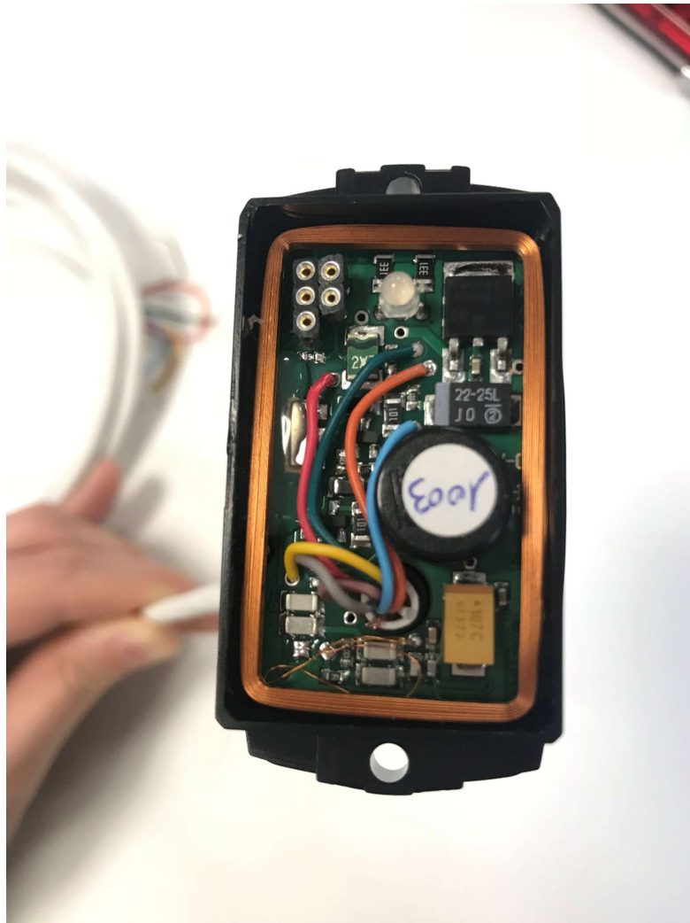
Motherboard integrated in the plastics before resin coating
