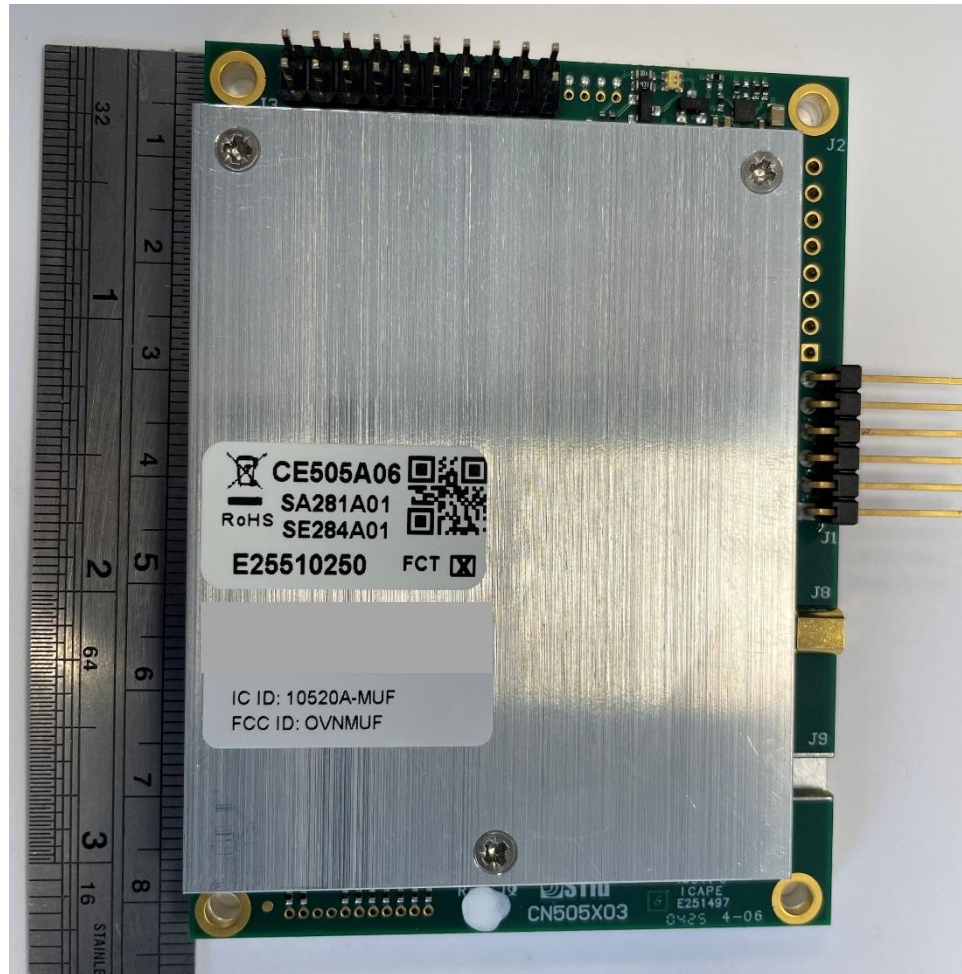
MUF electronic board with CEM shielding – Top side
