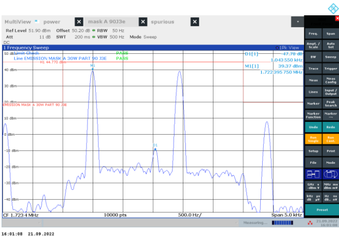
Figure 8.4-1: Low channel 30W 400 Hz and 1800 Hz 40 dB Carrier suppression
