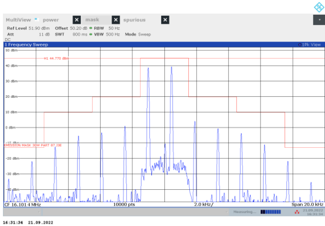
Figure 8.4-5: Mid channel 30W 1500 Hz 6 dB
