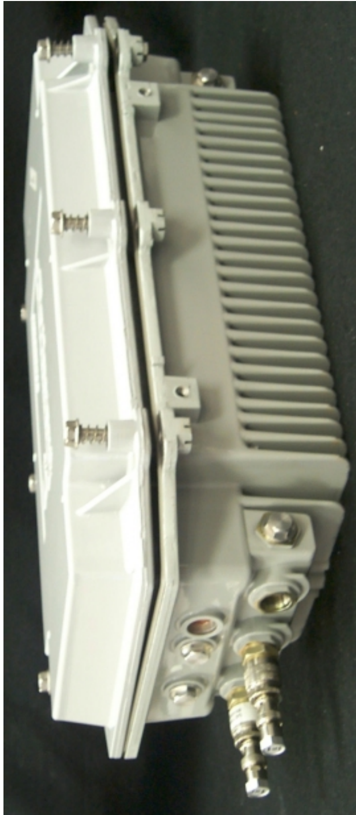
Photo 1. Front View of RF Network Amplifier
