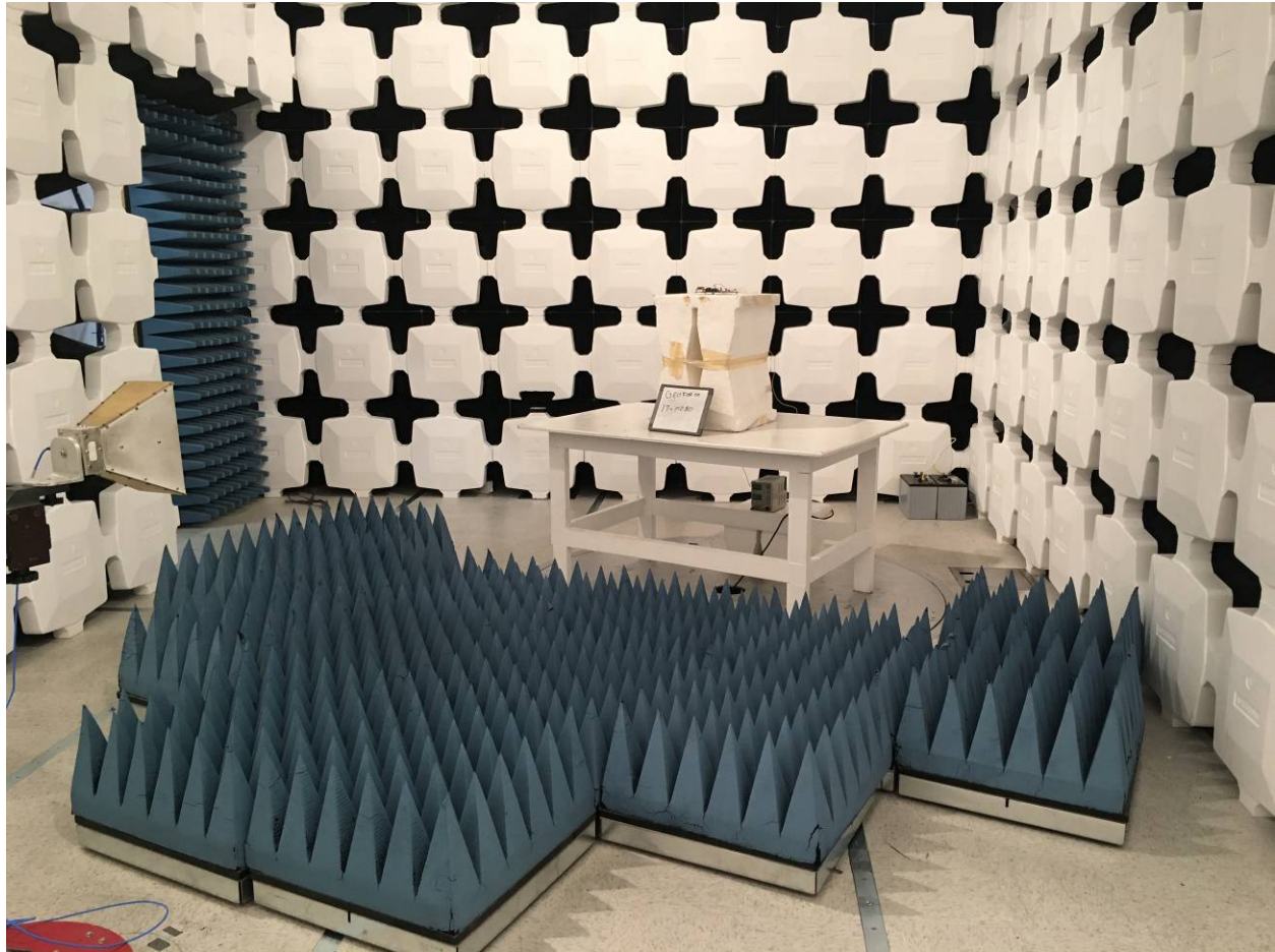
Figure 5. Test Configuration - above 1 GHz
