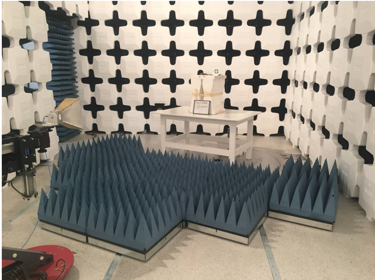
Figure 6. Test Configuration - above 1 GHz (External Antenna)
