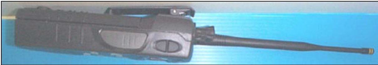
Figure 1. Handset positioned in the “Clip parallel” to phantom surface position.
