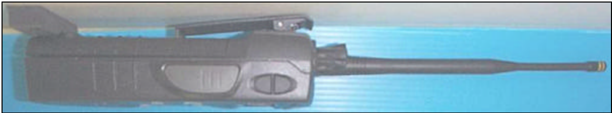
Figure 2. Handset positioned in the “Phone parallel” to phantom surface position
