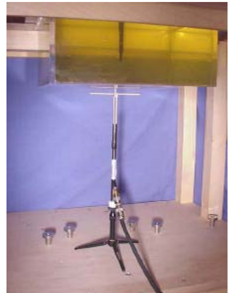
900MHz Dipole Validation Setup
