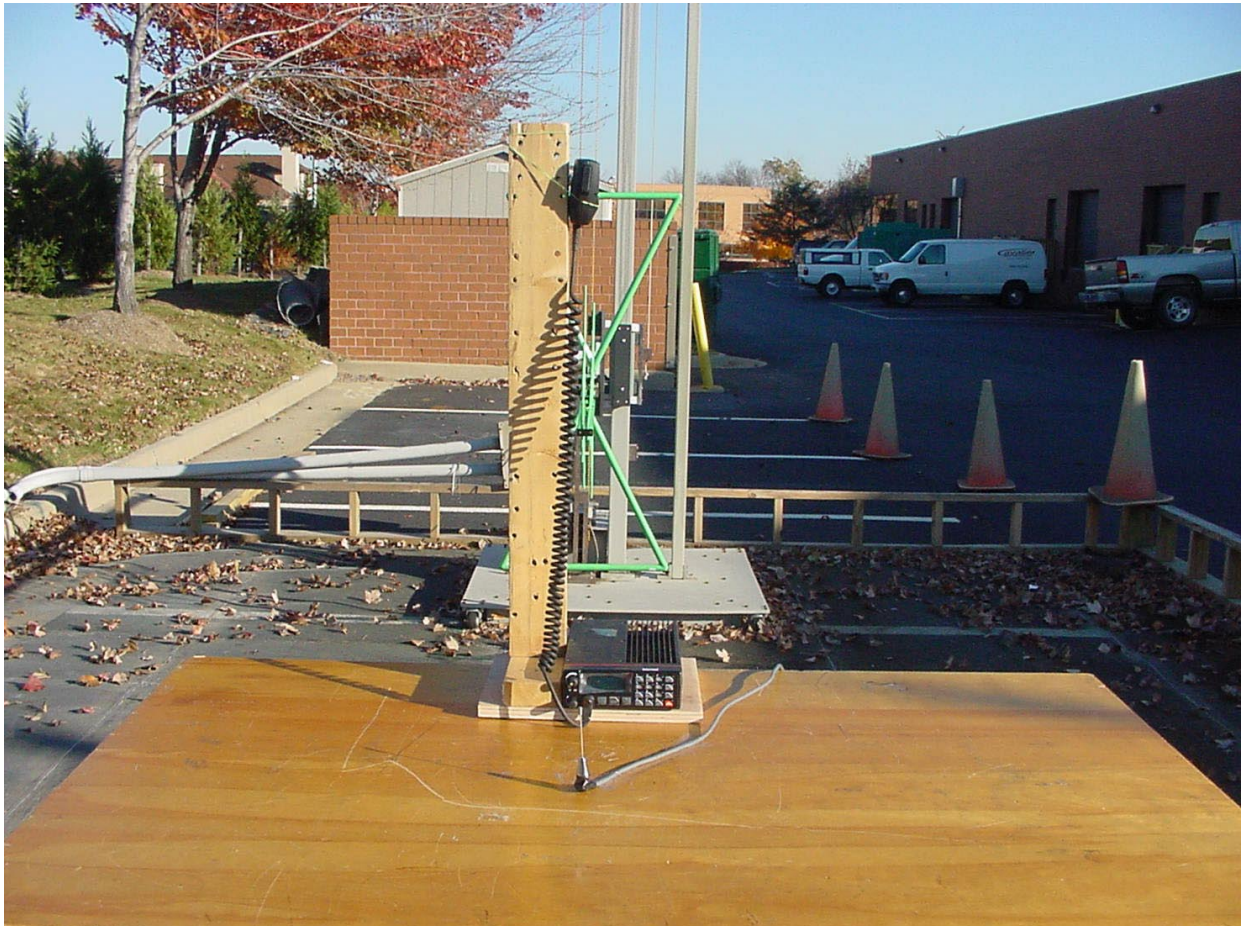
PHOTOGRAPH 1: RADIATED EMISSIONS FRONT VIEW
