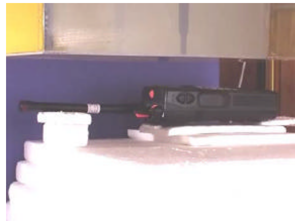
2.5cm Separation Distance - Antenna #2 (150-162MHz)
