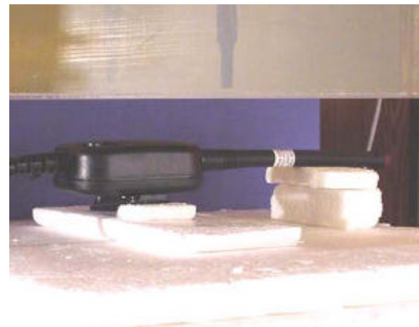
2.5cm Separation Distance - Antenna #2 (150-162MHz)
