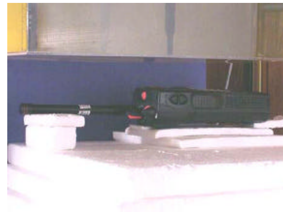
2.5cm Separation Distance - Antenna #3 (162-174MHz)
