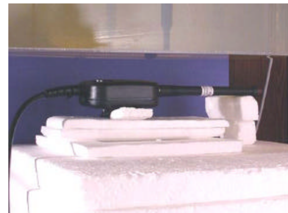
2.5cm Separation Distance - Antenna #3 (162-174MHz)
