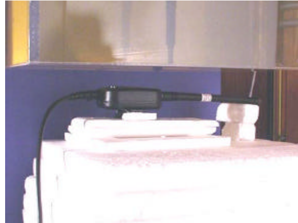
2.5cm Separation Distance - Antenna #1 (136-151MHz)
