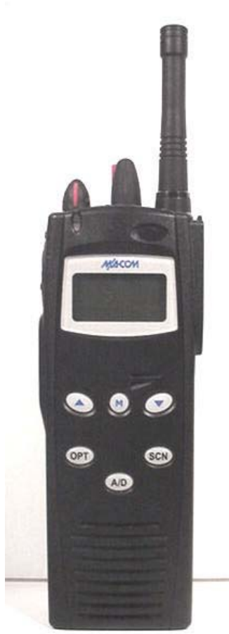
EUT (P/N: T1-HSAR01) with Helical Coil Antenna (P/N: KRE1011219/10)
