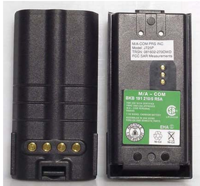
Nickel Cadmium Battery – Intrinsically Safe (P/N: BKB191210/5)
