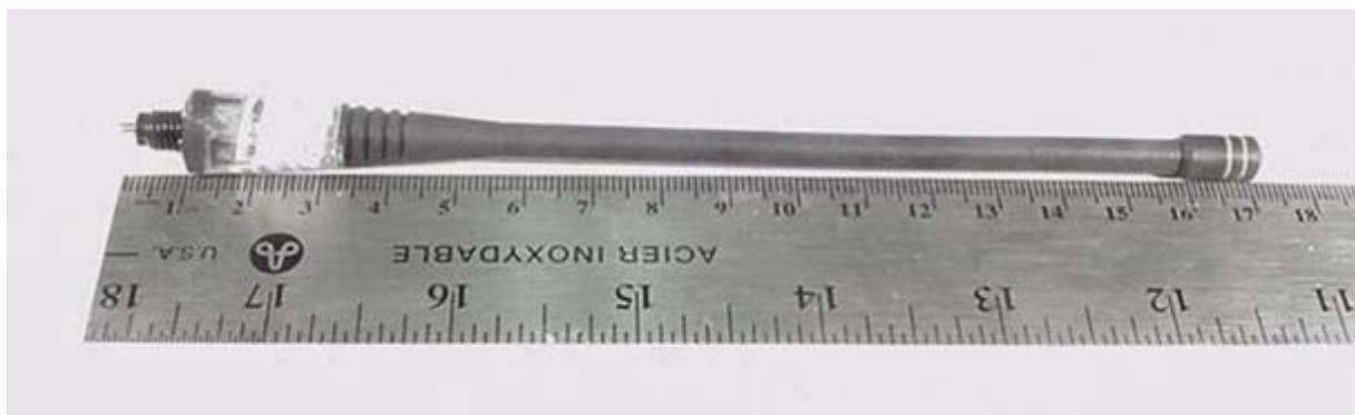
Spring Whip Antenna – 378-430 MHz (P/N: KRE1011223/10)
