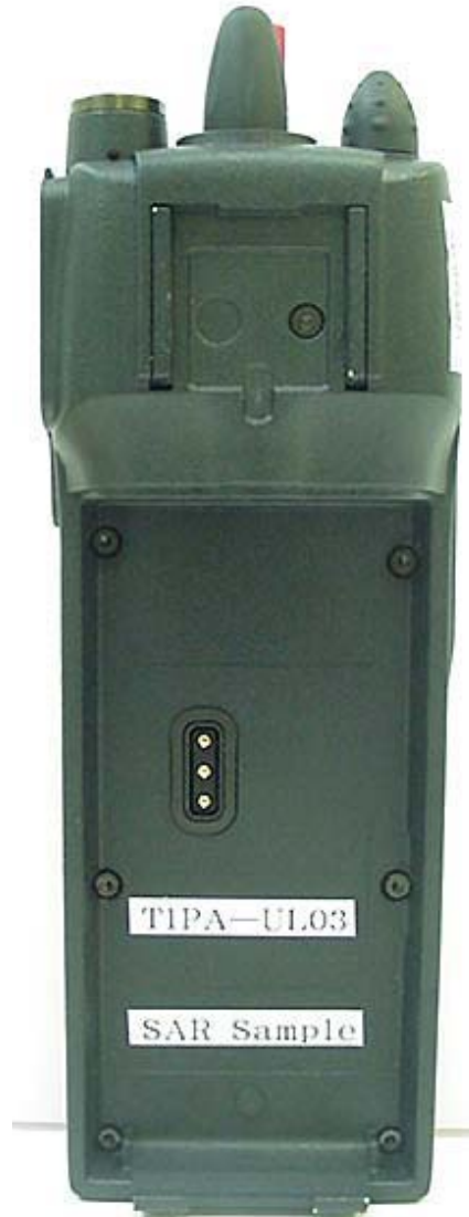
DUT Battery Compartment (S/N: T1PA-UL03) P/N: RU101219V61 R1B (Scan)
