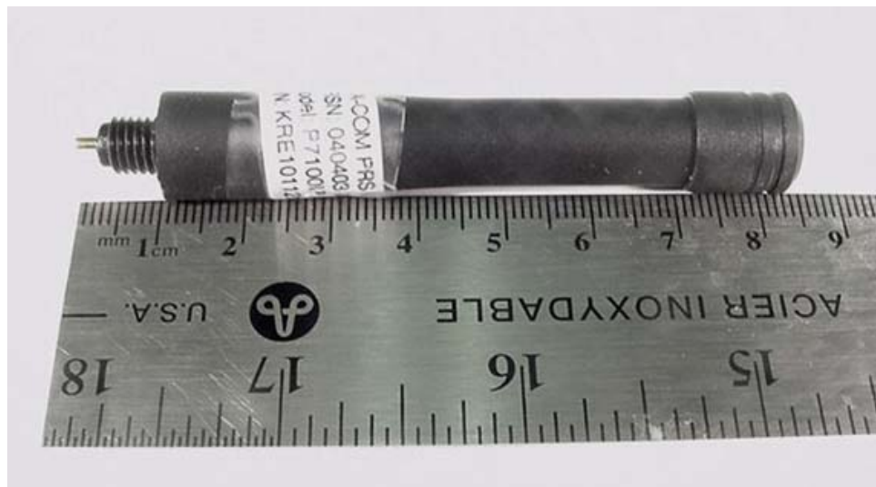
Helical Coil Antenna - 403-430 MHz (P/N: KRE1011219/10)
