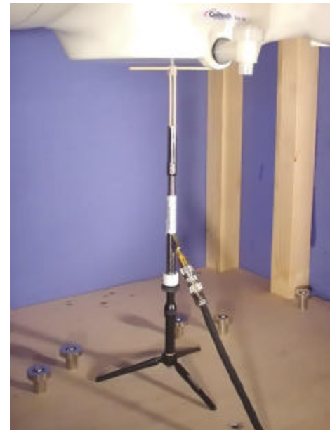
900MHz System Check Setup Photograph
