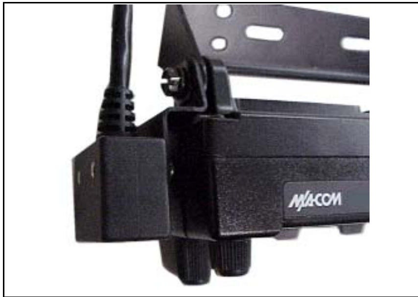
Figure 9-10: Pigtail Bracket Installed on Control Unit
