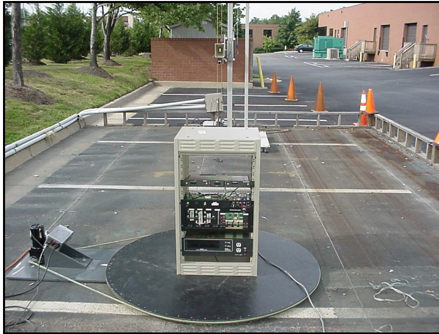
PHOTOGRAPH 1: RADIATED EMISSIONS FRONT VIEW
