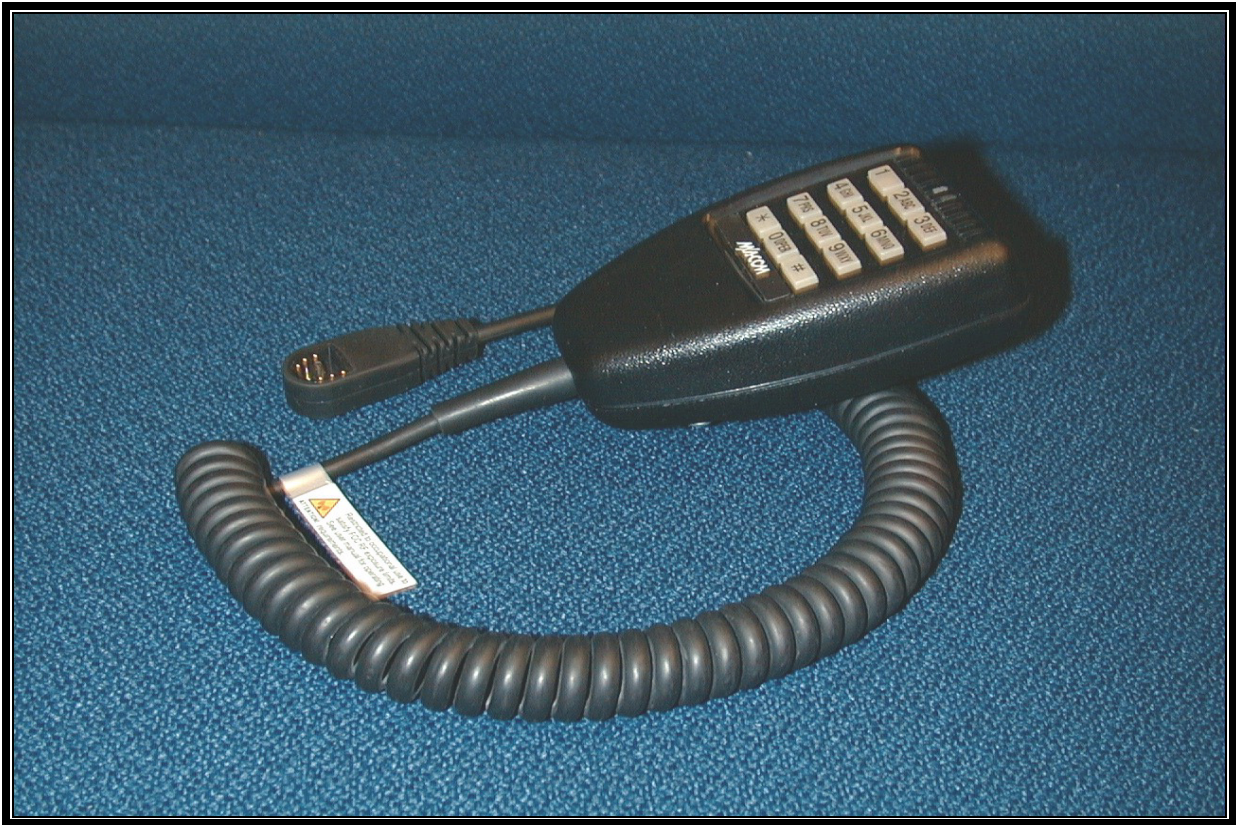
PHOTOGRAPH 5: DTMF MICROPHONE WITH RF LABEL
