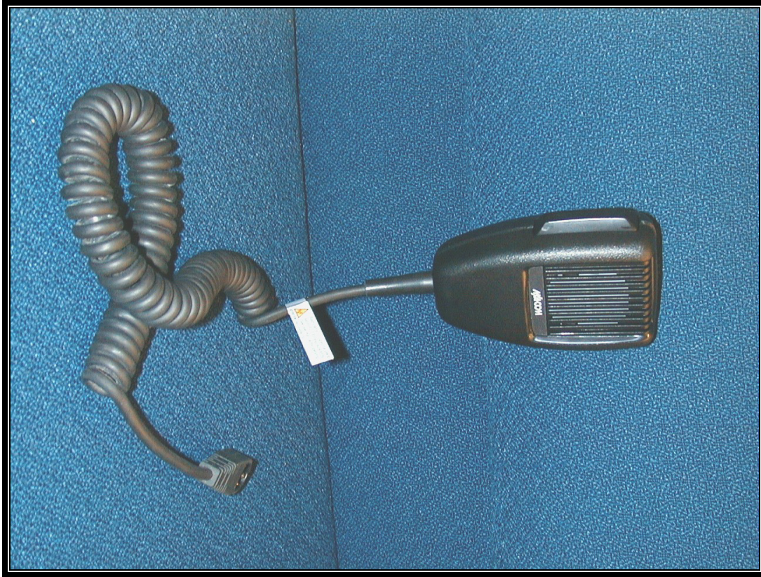
PHOTOGRAPH 7: NOISE CANCELLATION MICROPHONE WITH RF LABEL
