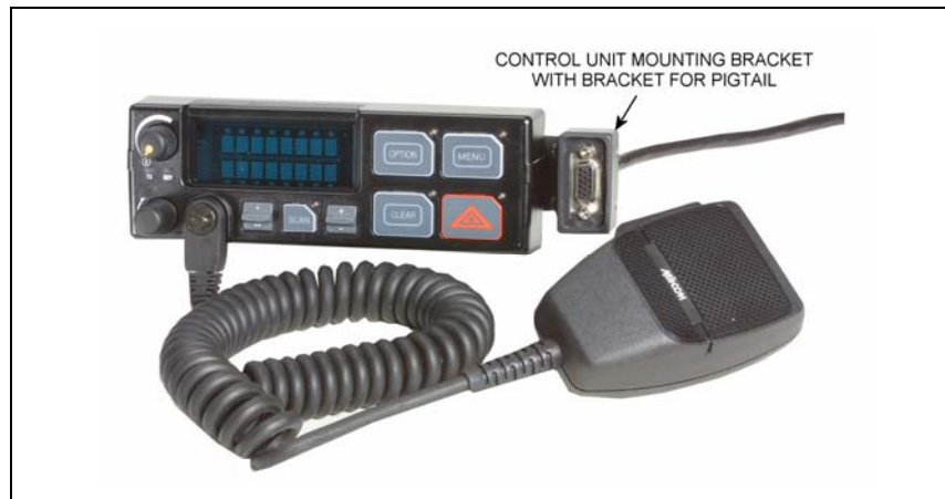
Figure 9-8: Control Unit Mounting Bracket with Pigtail Bracket
