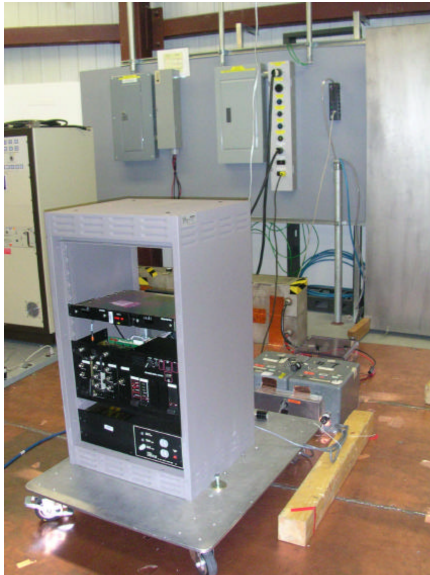
Figure 8-2: Conducted Emissions Test Set-Up
