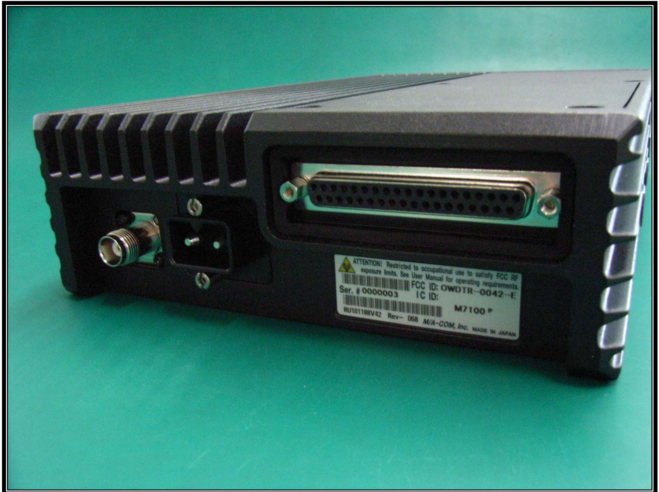
Photograph 2: Label Location on Rear of M7100
