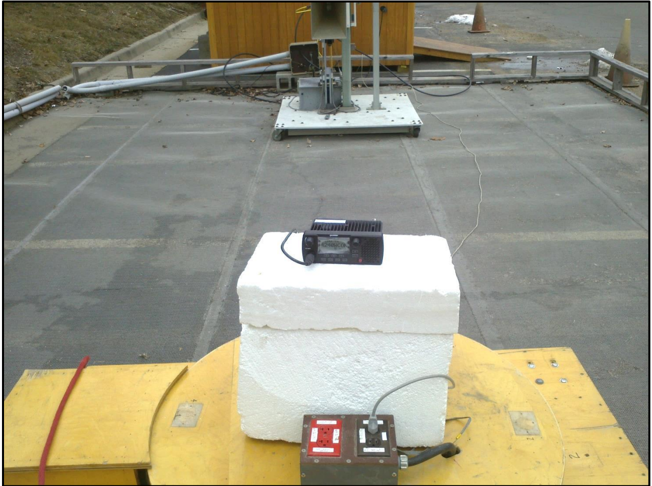
Photograph 1: Radiated Emissions – Front View
