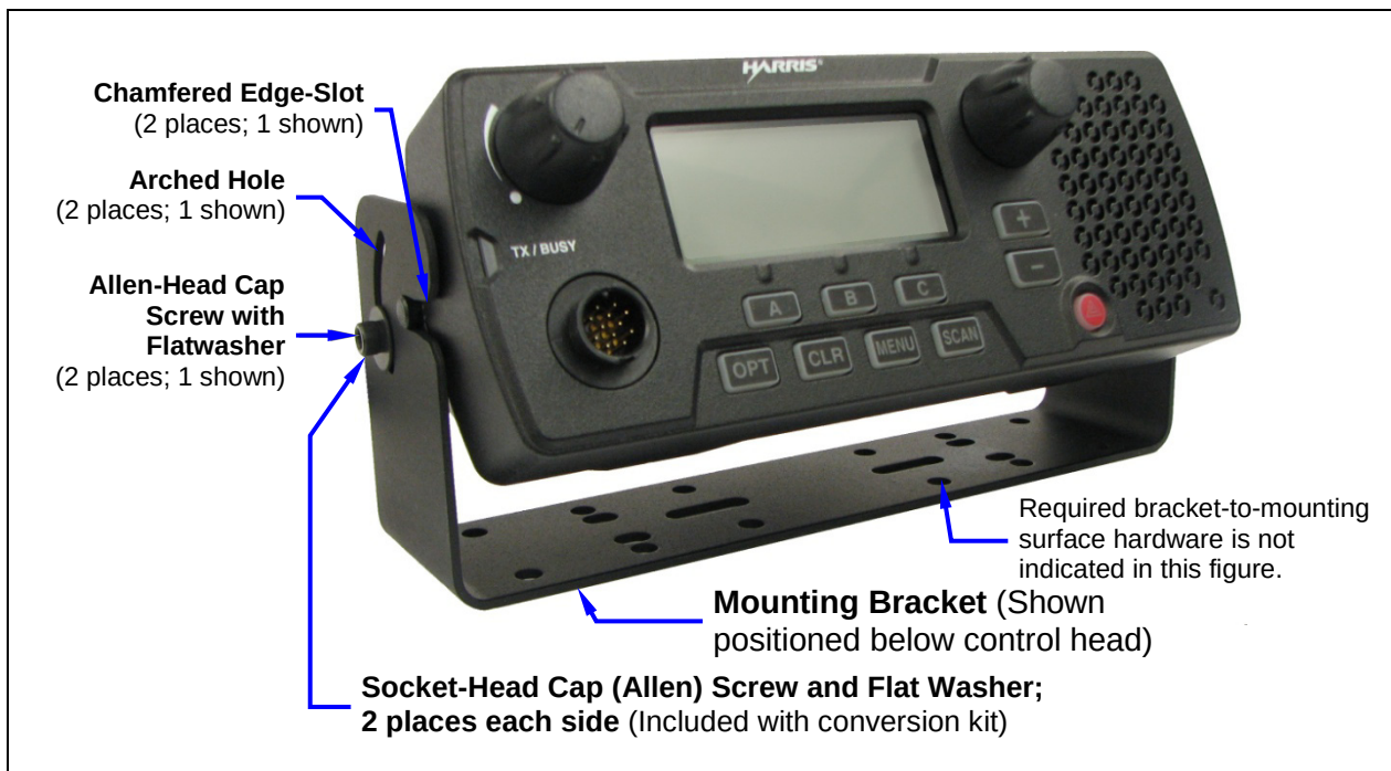
Figure 8-1: Control Head Mounting Bracket (shown positioned below head)
