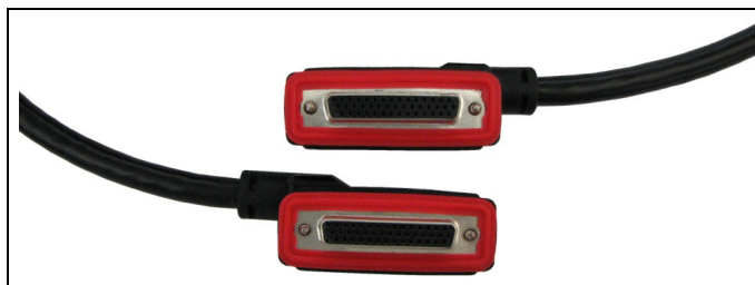
Figure 8-2: D-Shaped Connectors of Remote Control Cable
