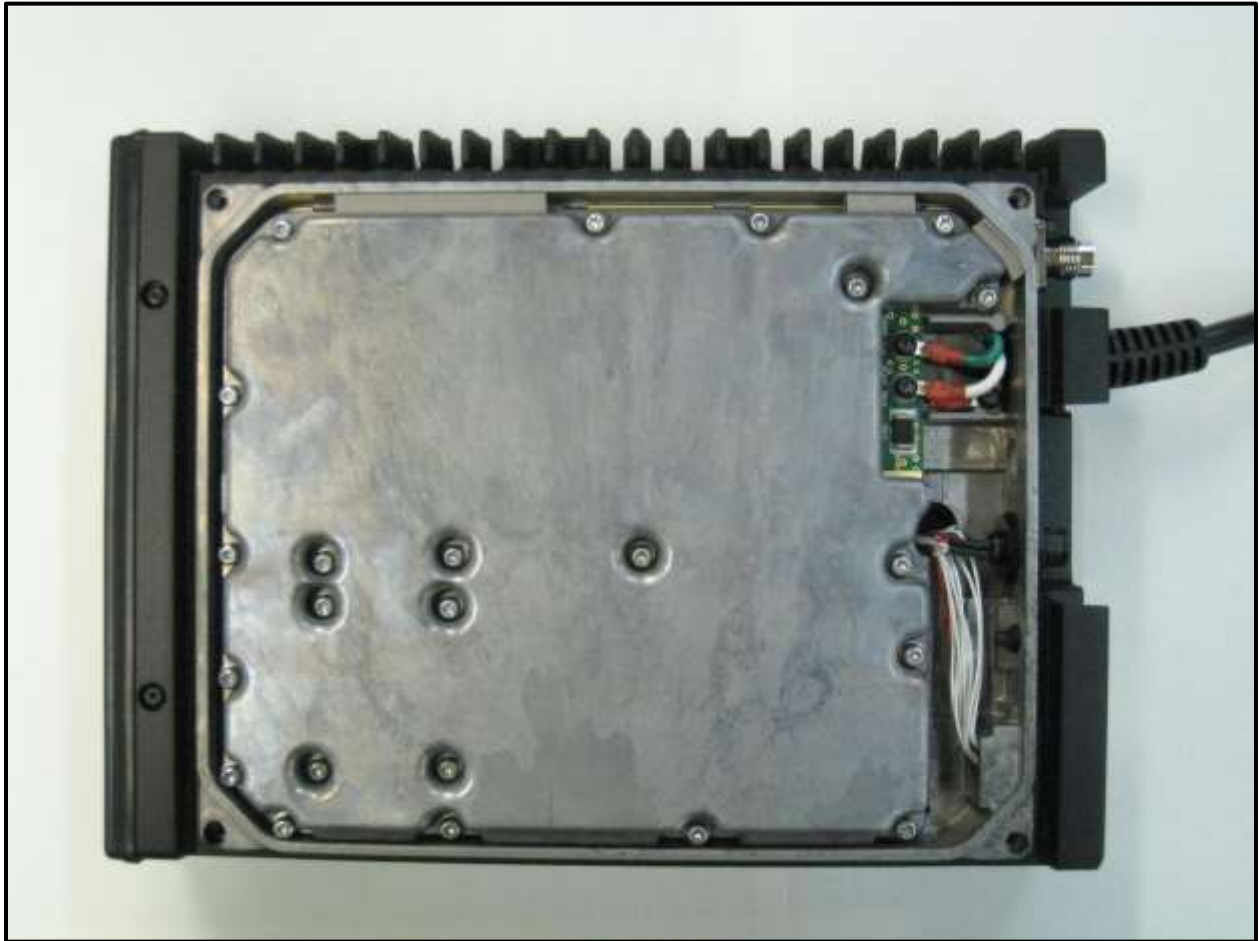
Photograph 19: Bottom Cover Removed
