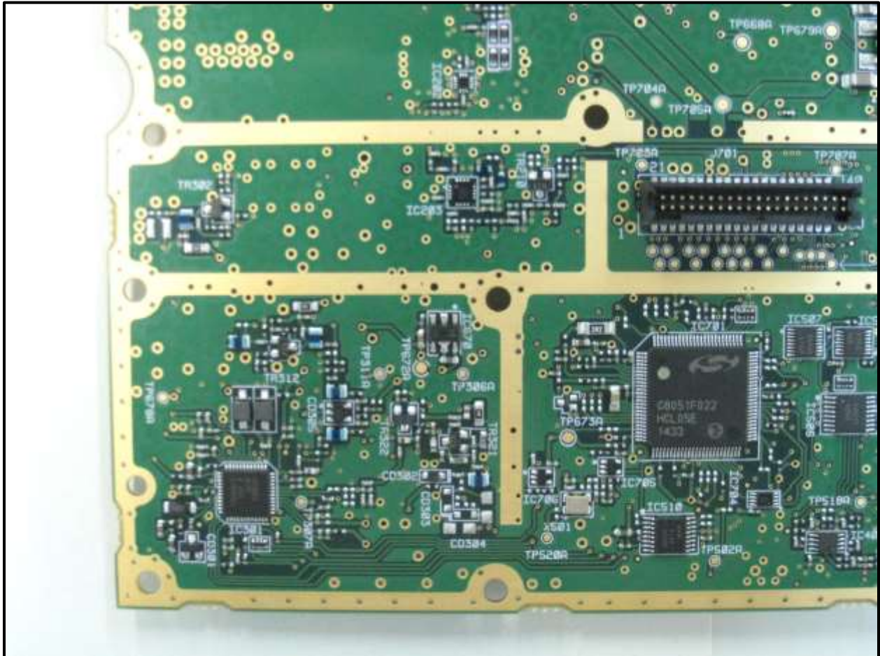
Photograph 29: RF Processor – Solder Side; Lower Left
