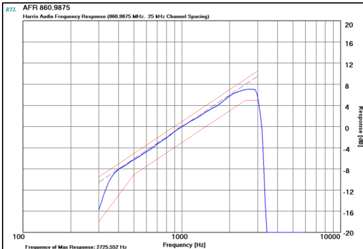
Plot 10-4: Modulation Characteristics - Audio Frequency Response – 860.9875 MHz; WB
