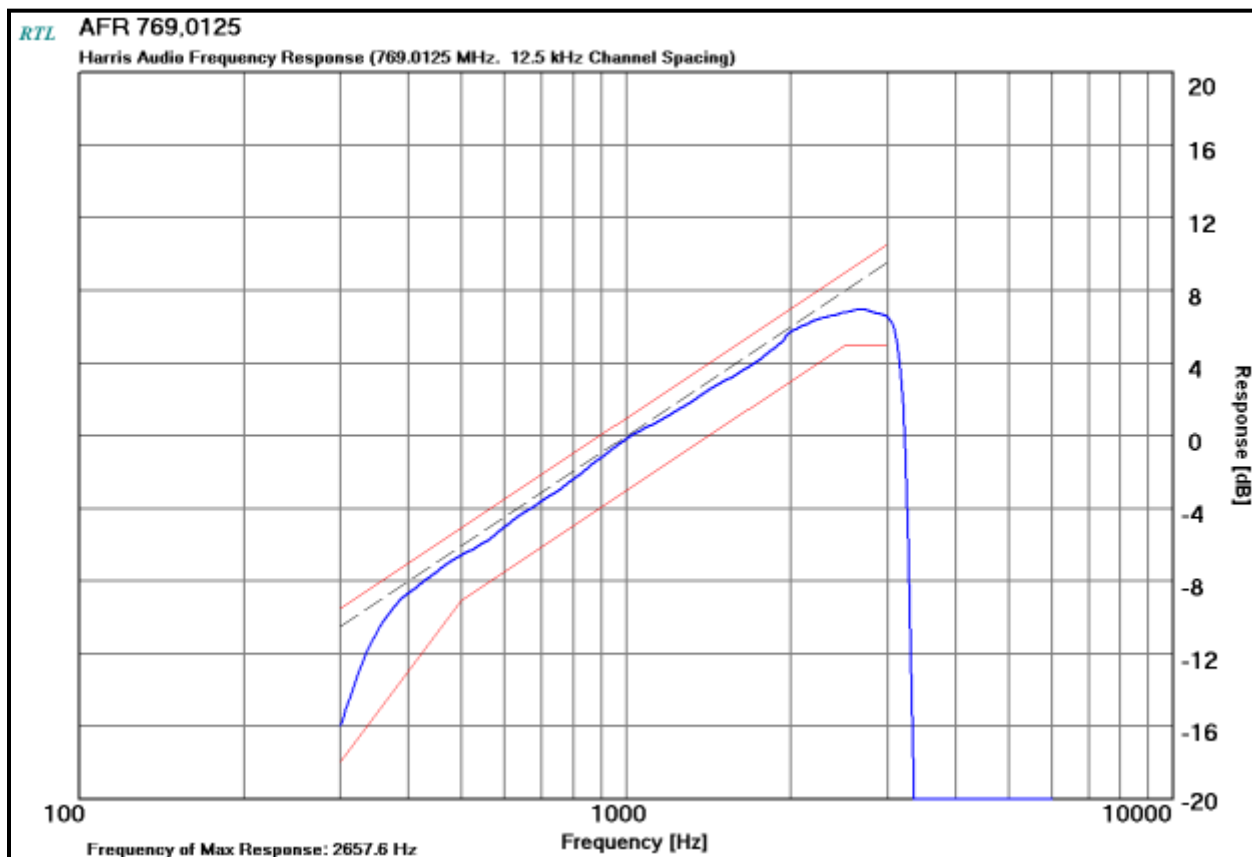
Plot 10-1: Modulation Characteristics - Audio Frequency Response – 769.0125; MHz NB
