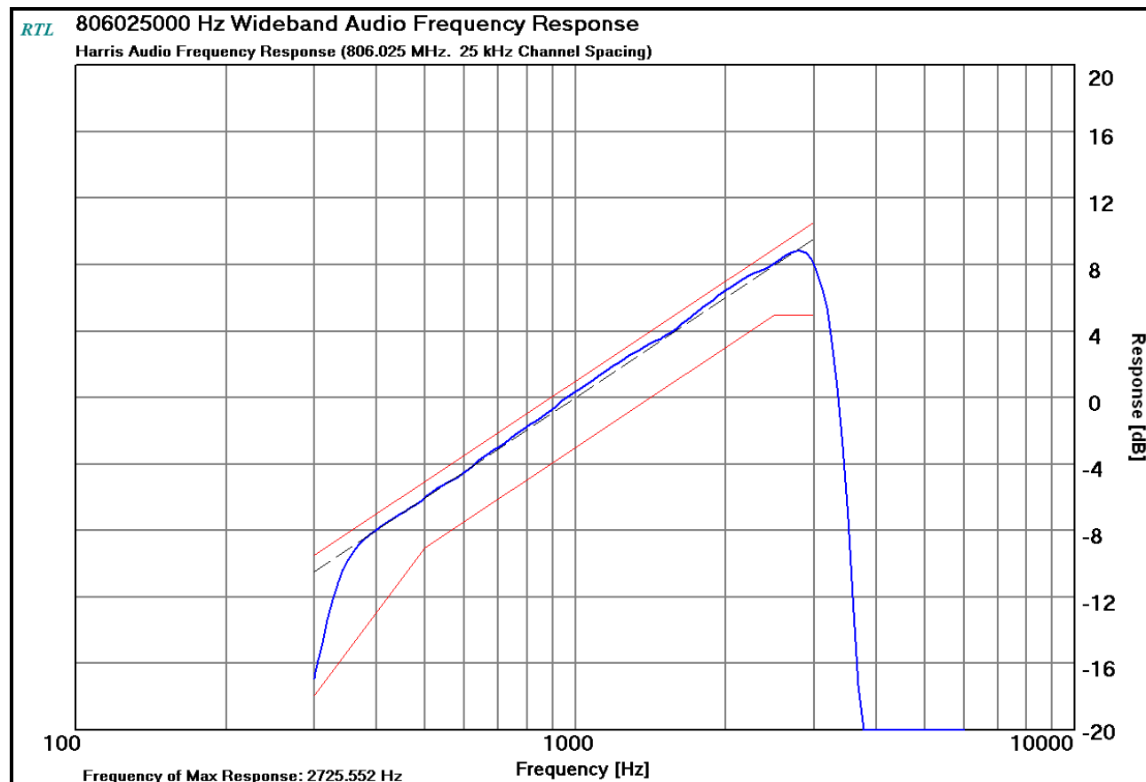
Plot 10-10: Modulation Characteristics - Audio Frequency Response – 806.0250 MHz
