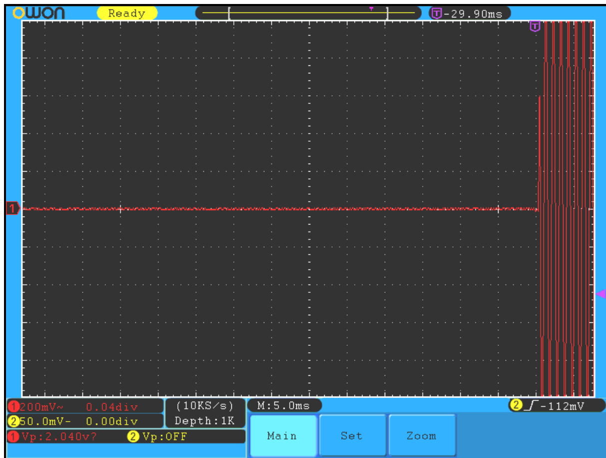
Plot 11-16: Transient Frequency Behavior – 173.9875 MHz; Narrow Band; Carrier OFF Time
