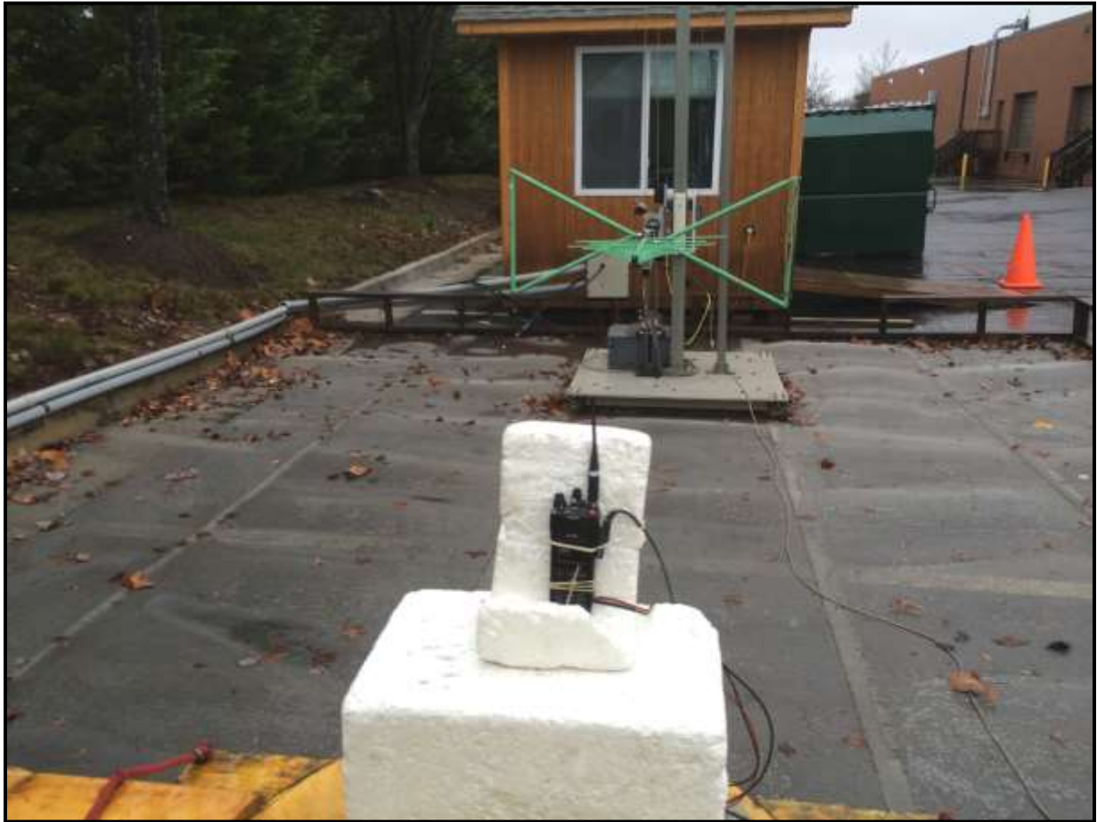
Photograph 3: Radiated Emissions Testing – Front View <1 GHz
