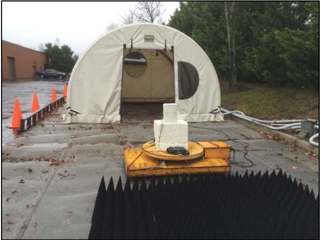
Photograph 2: Radiated Emissions Testing – Back View >1 GHz
