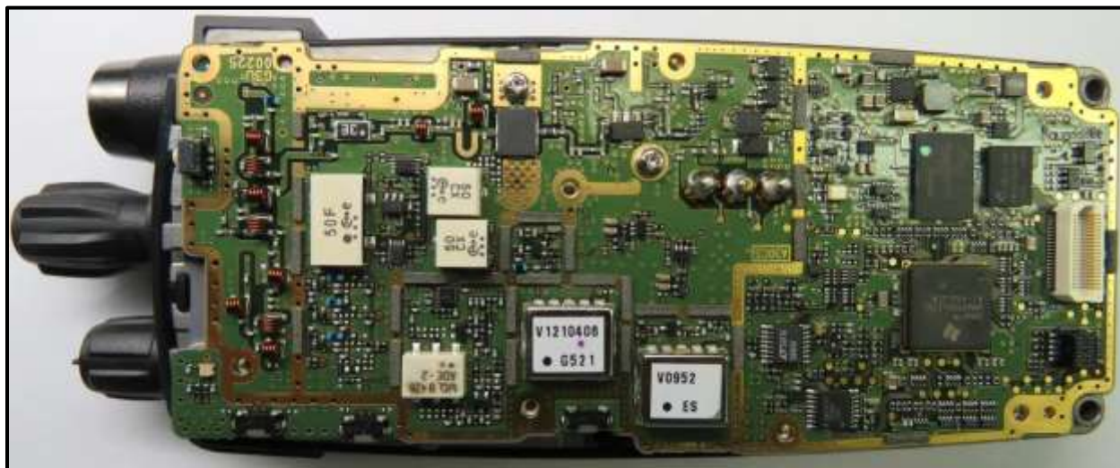
Photograph 16: Main PWB in Unit without Shield
