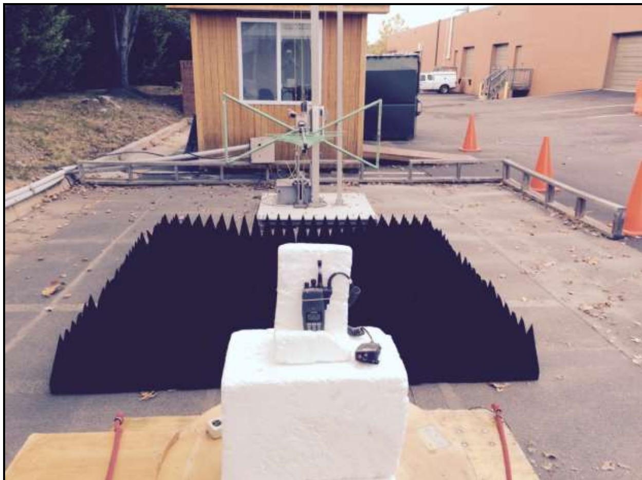
Photograph 4: Radiated Emissions (Spurious/Harmonics) – Front View above 1 GHz
