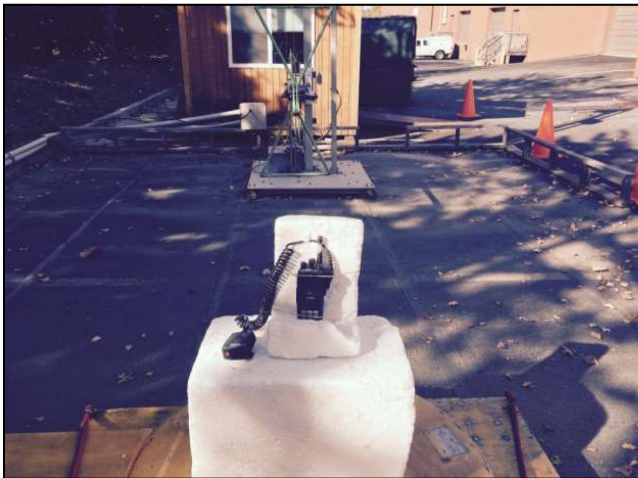
Photograph 2: Radiated Emissions (Spurious/Harmonics) – Front View below 1 GHz
