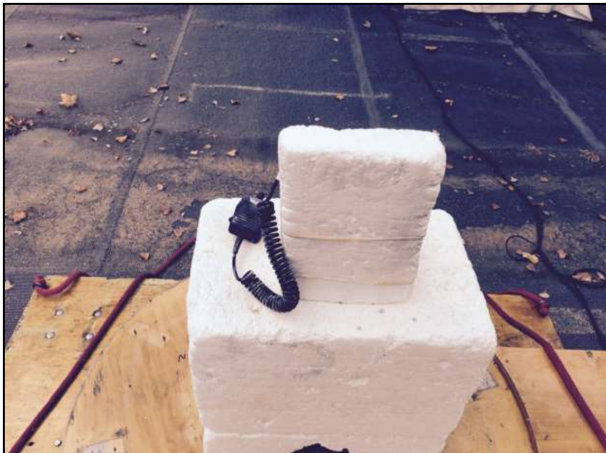
Photograph 5: Radiated Emissions (Spurious/Harmonics) – Back View above 1 GHz
