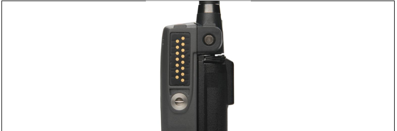
Figure 5-2: XG-15P 15-Pin Universal Device Connector
