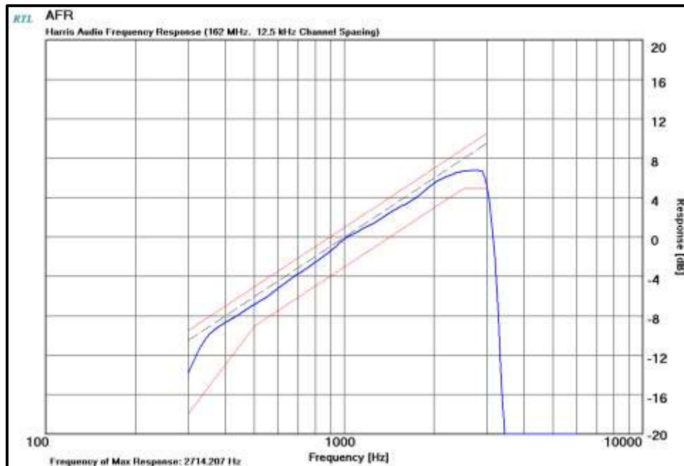
Plot 9-1: Modulation Characteristics - Audio Frequency Response – 162.0000 MHz
