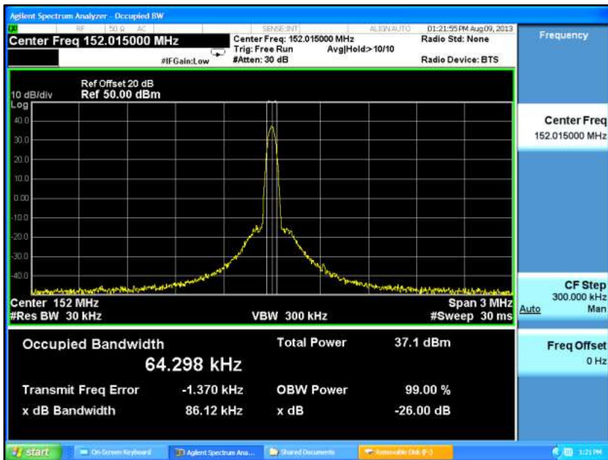
Plot 7-48: Occupied Bandwidth – NB Analog
