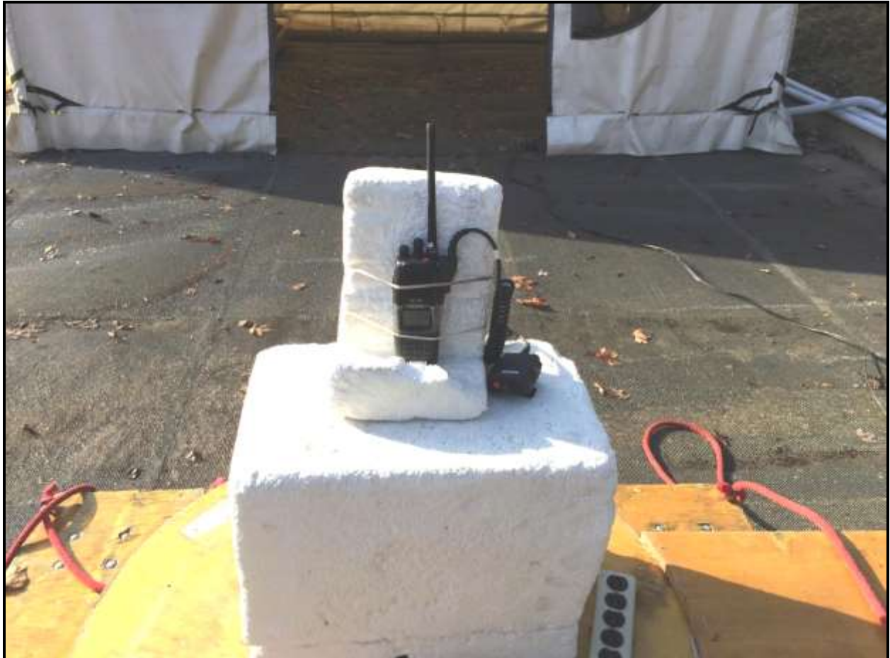
Photograph 1: Radiated Emissions – Front View
