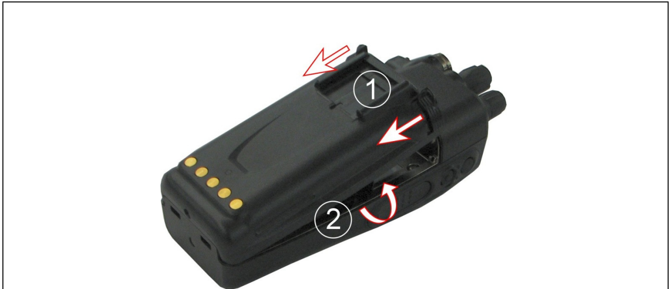
Figure 4-1: Removing the Battery Pack
