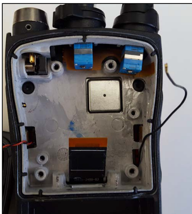
Expansion Board Removed
