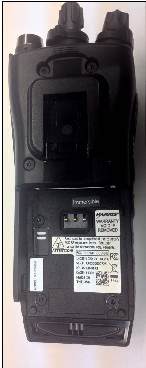
ID Label Location & RF Exposure Statement on Back of EUT
