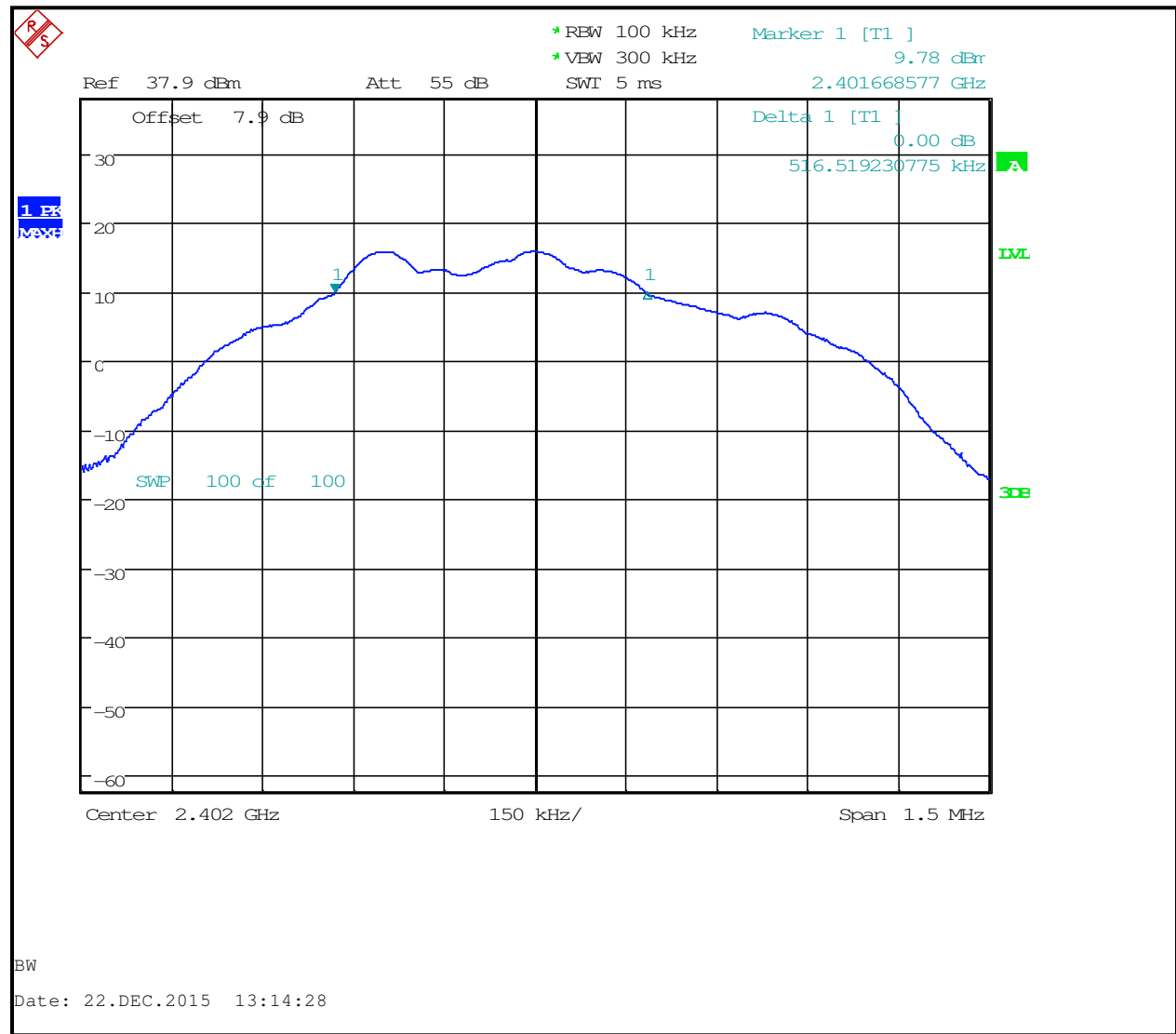
Plot 7-1: 6 dB Bandwidth – 2402 MHz
