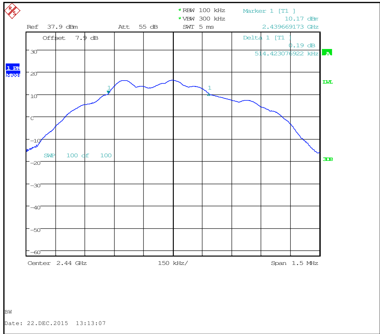
Plot 7-2: 6 dB Bandwidth – 2440 MHz
