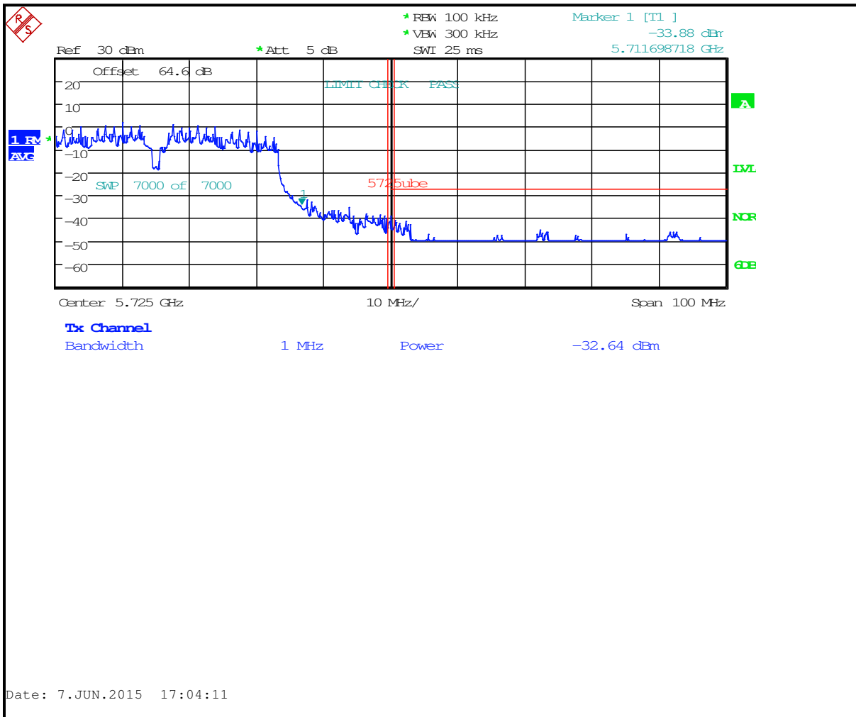
Plot 6-32: Upper Band Edge: Measurement Channel 140 (5700 MHz, 40 MHz BW, 802.11n, Average)
