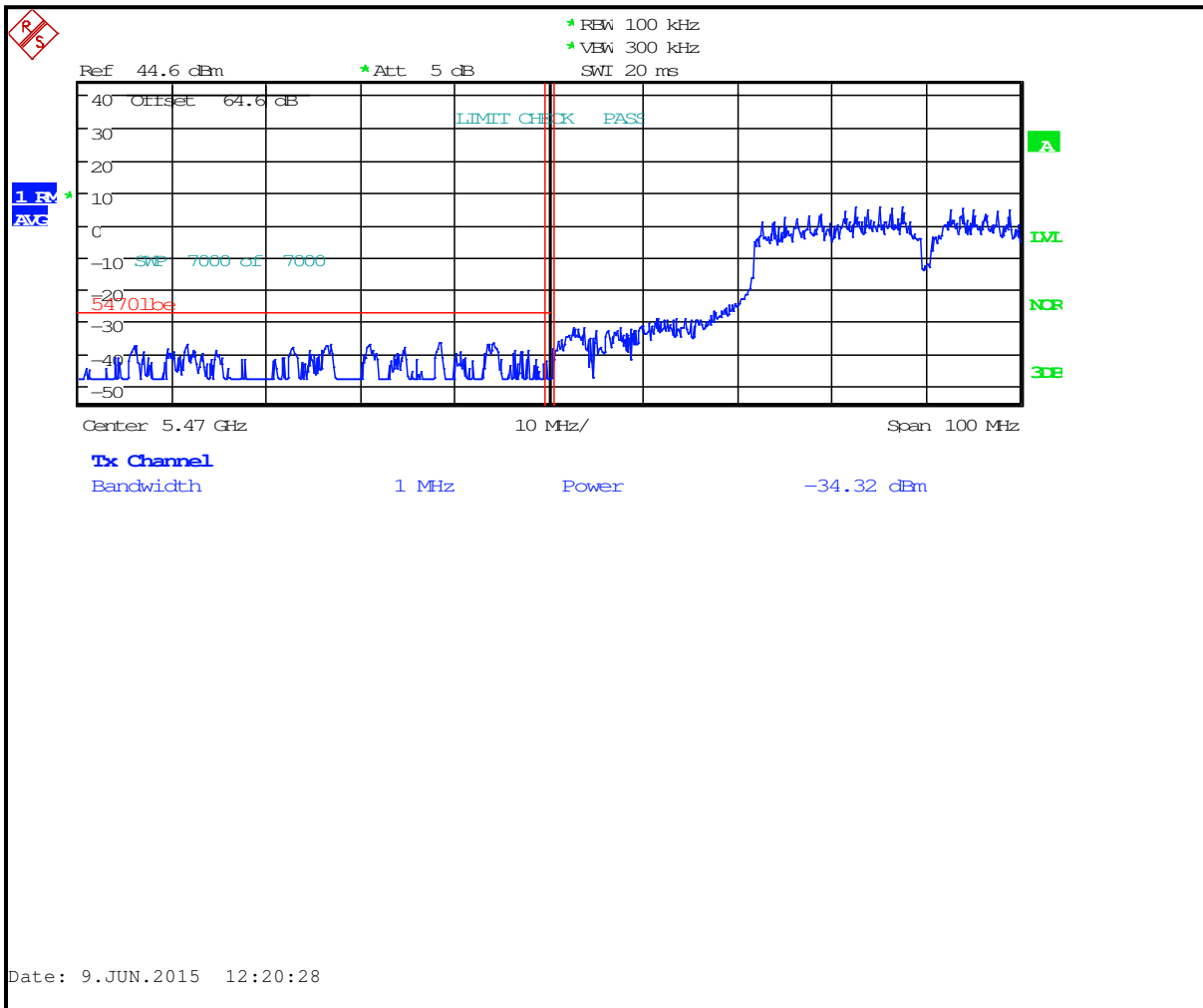
Plot 6-22: Lower Band Edge: Measurement Channel 100 (5500 MHz, 40 MHz BW, 802.11a, Average)
