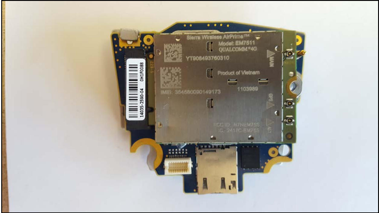
Expansion Board with LTE Module and LTE Processor Shield - Top
