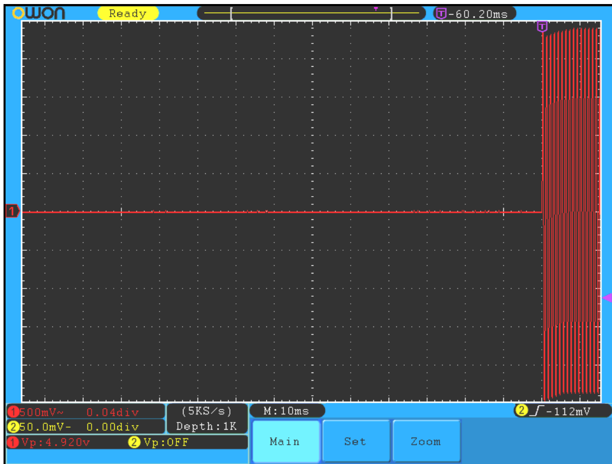
Plot 11-18: Transient Frequency Behavior – 430.0125 MHz; Wide Band; Carrier OFF Time
