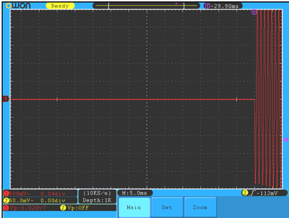
Plot 11-10: Transient Frequency Behavior – 162.0125 MHz; Wide Band; Carrier OFF Time
