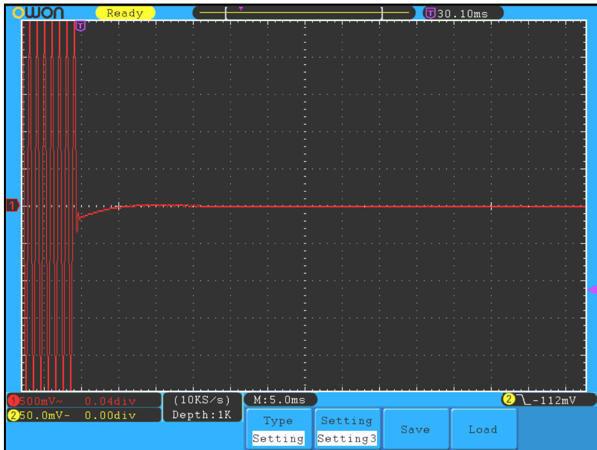
Plot 11-1: Transient Frequency Behavior – 150.0125 MHz; Wide Band; Carrier ON Time
