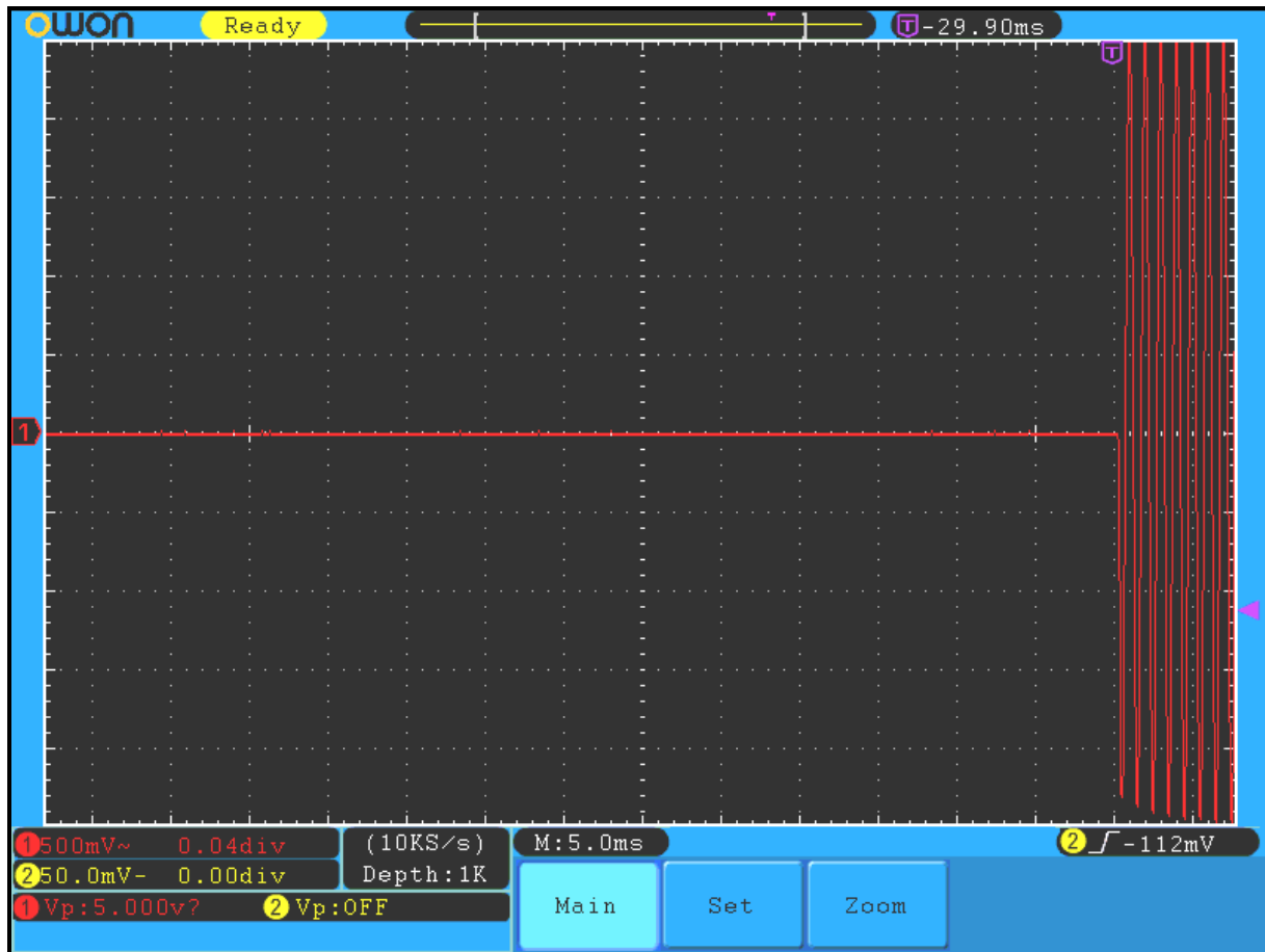
Plot 11-14: Transient Frequency Behavior – 173.9875 MHz; Wide Band; Carrier OFF Time
