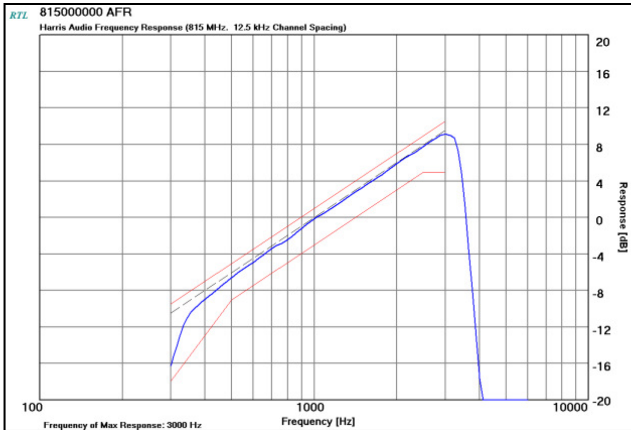
Plot 10-11: Modulation Characteristics - Audio Frequency Response – 815.0000 MHz
