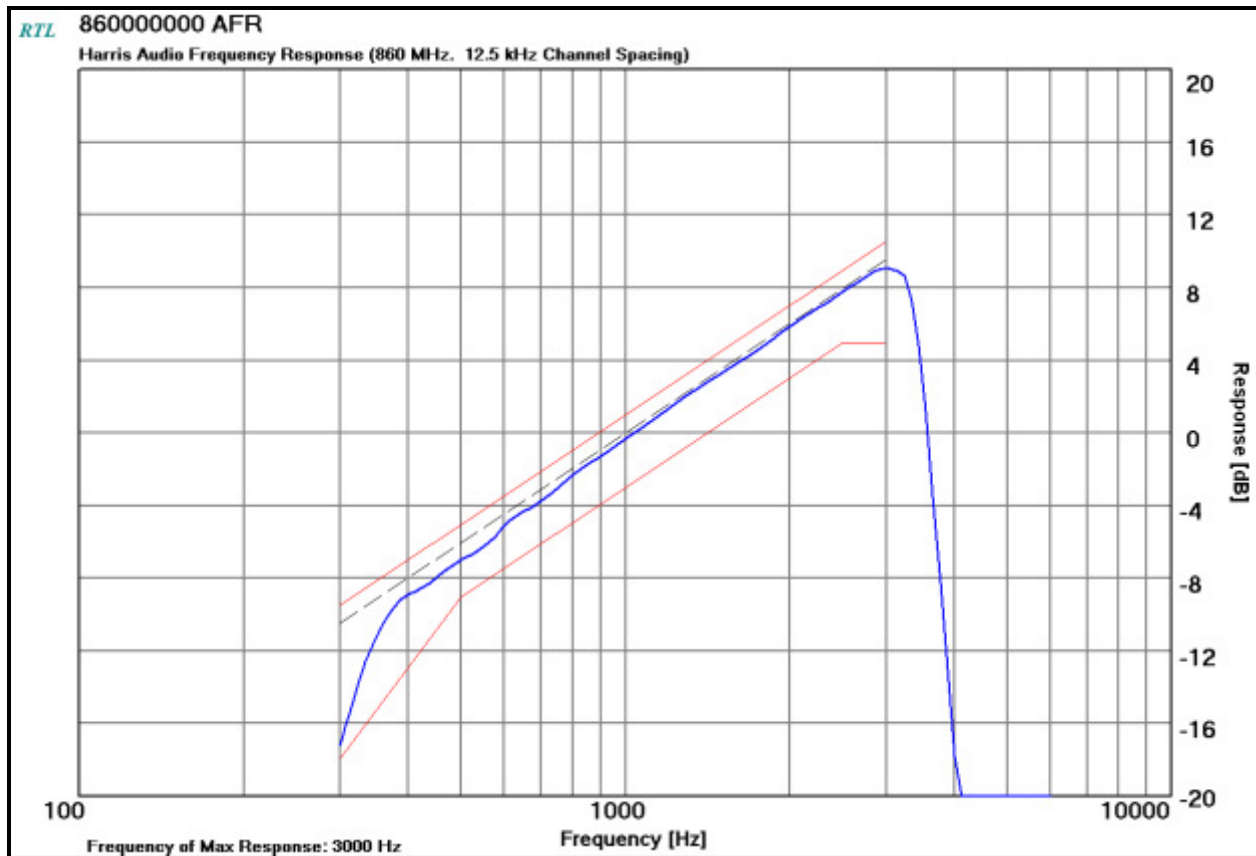
Plot 10-14: Modulation Characteristics - Audio Frequency Response – 860.0000 MHz
