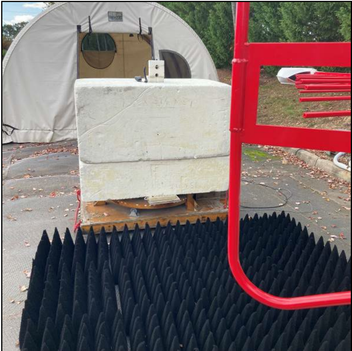
Photograph 2: Radiated Emissions (Spurious/Harmonics) Over 1 GHz, Back View
