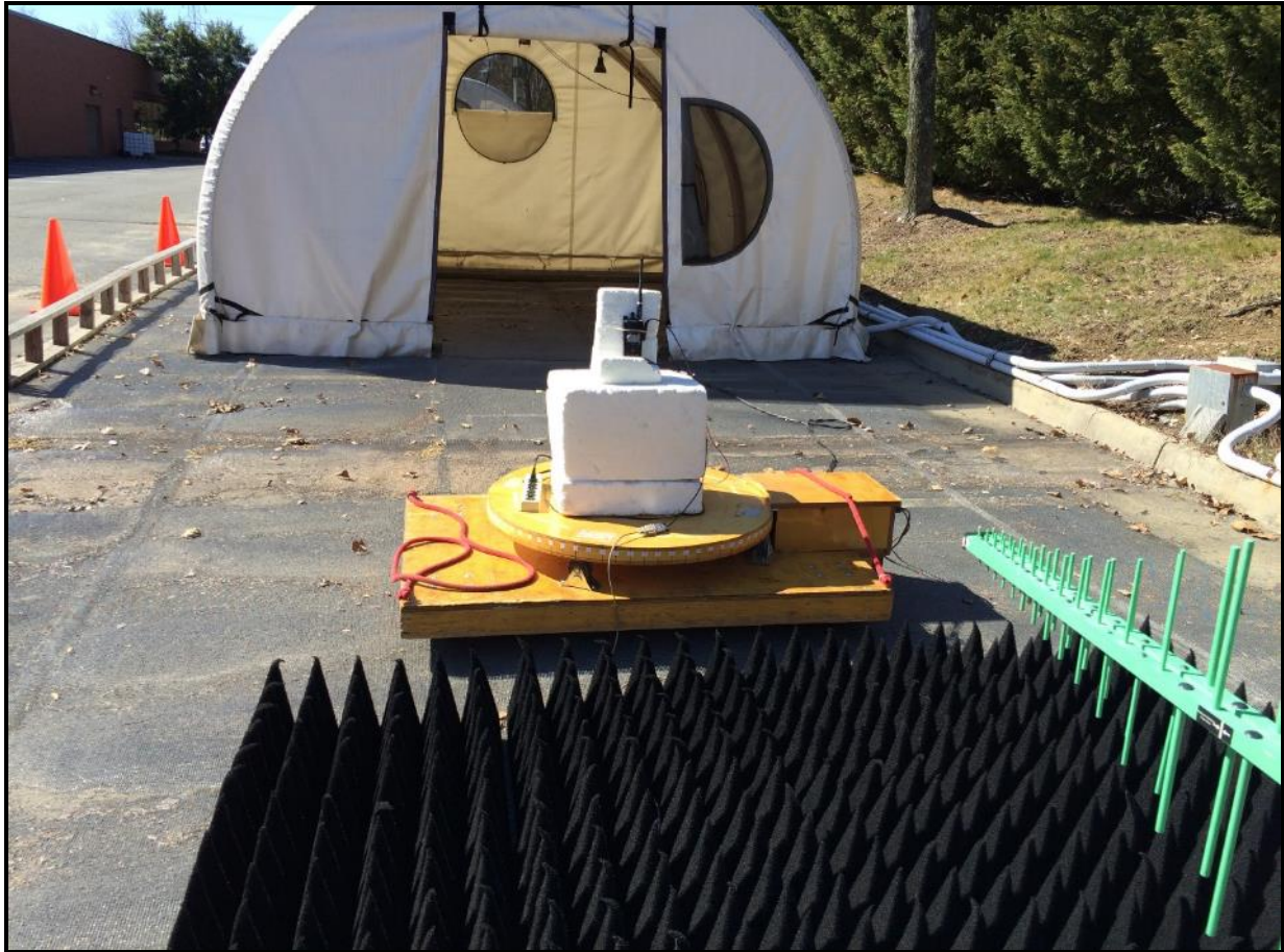
Photograph 1: Radiated Emissions Testing – Front View
