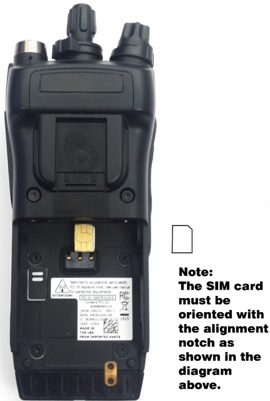
Figure 4-4: SIM Card Installation
