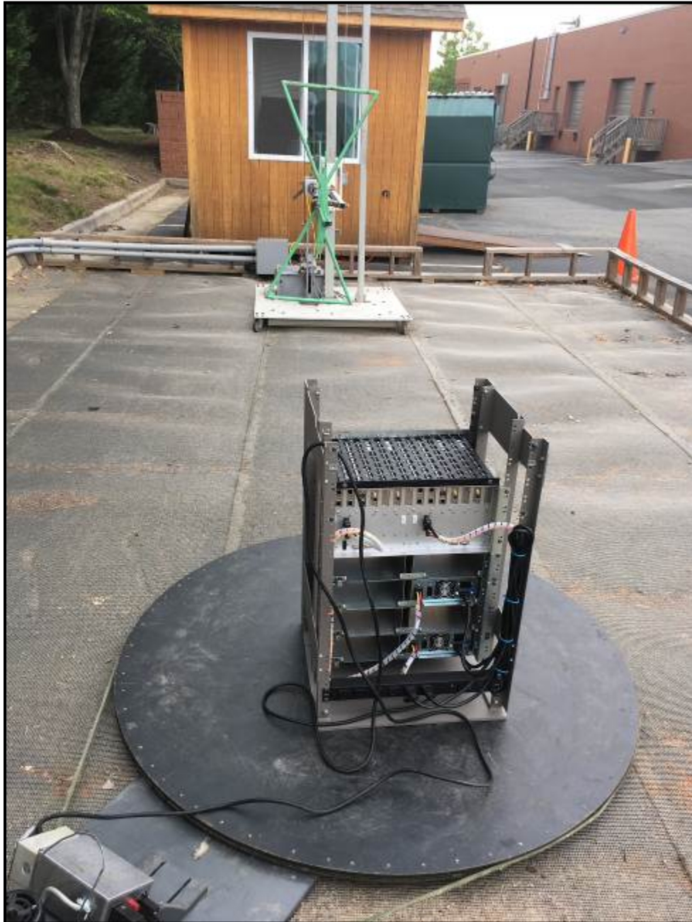
Photograph 2: Radiated Emissions (Spurious/Harmonics)
