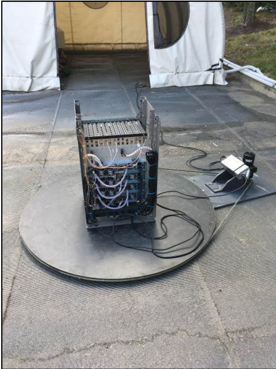
Photograph 4: Radiated Emissions (Spurious/Harmonics) – Back View (Below 1 GHz)
