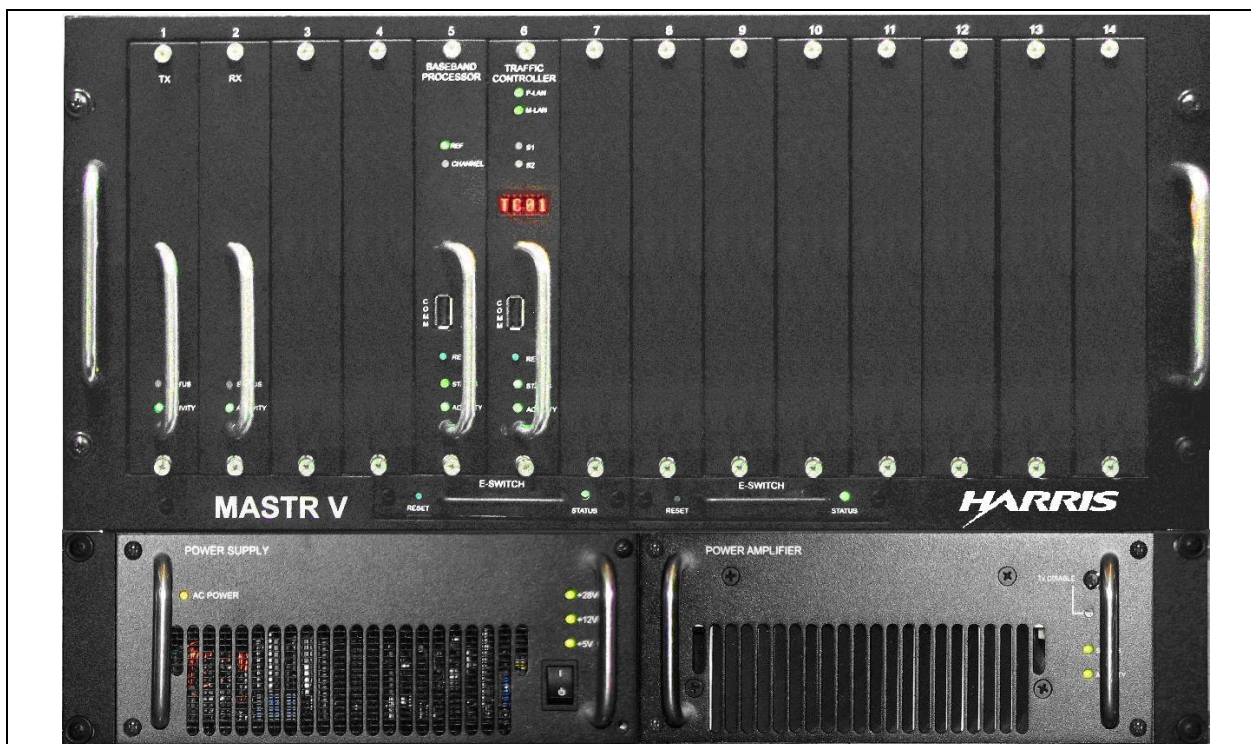
Figure 3-1: MASTR V Multi-Channel Base Station Shelf Equipped with One (1) RF Channel
