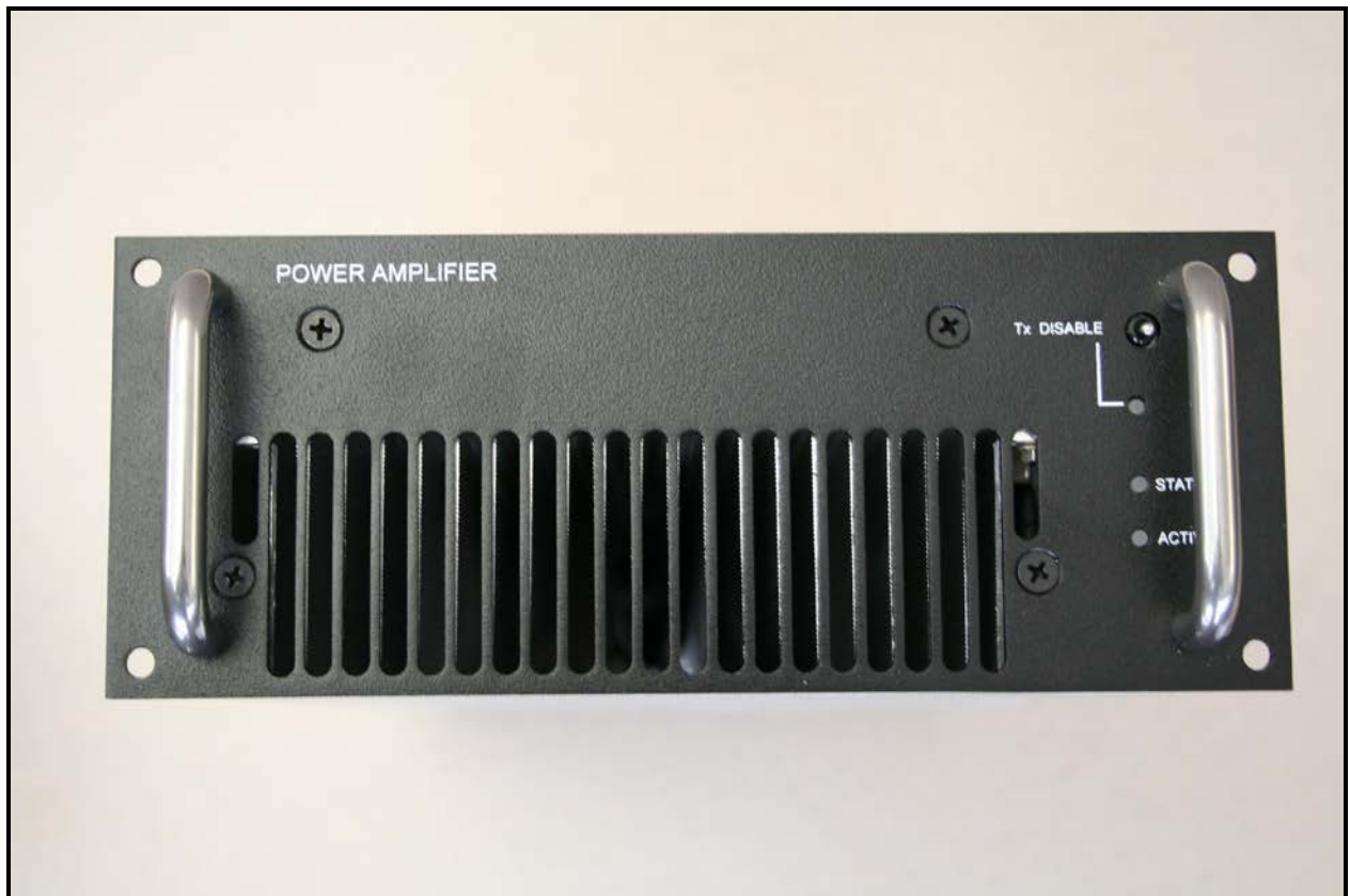
High Power Amplifier Front View
