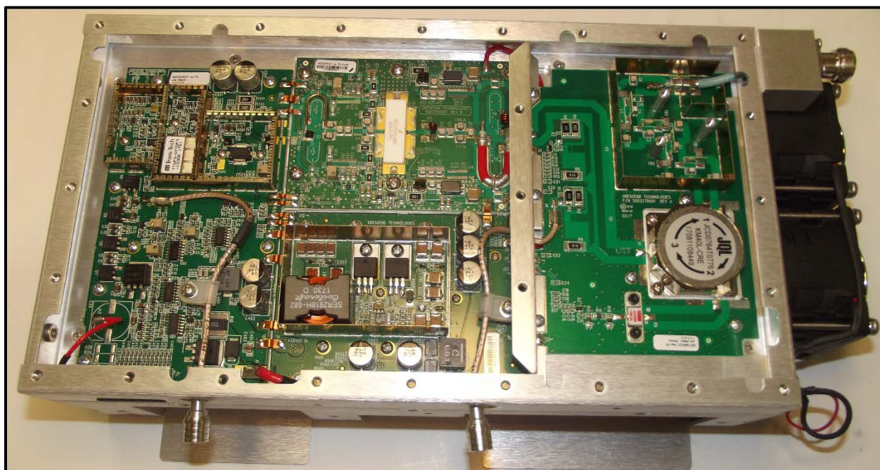
Power Amplifier Top View No Shields
