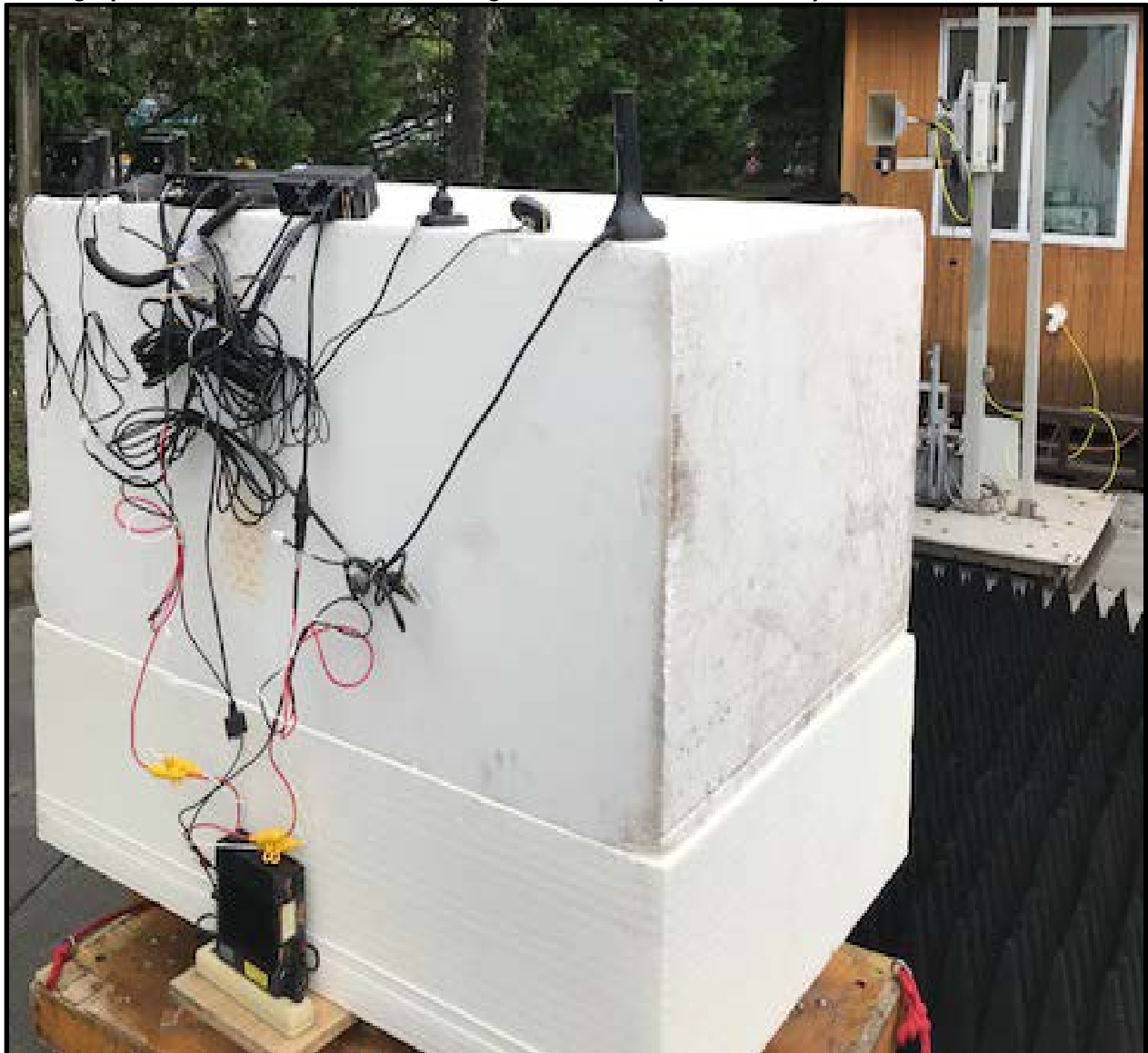
Photograph 2: Radiated Emissions Testing – Back View (Above 1 GHz)
