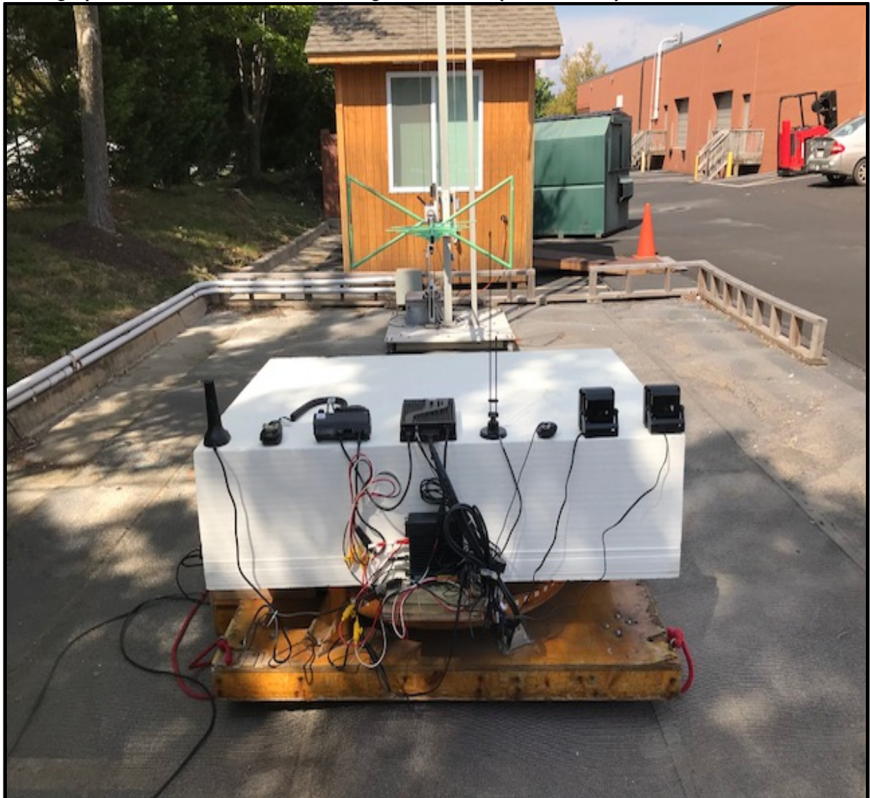
Photograph 4: Radiated Emissions Testing – Back View (Below 1 GHz)
