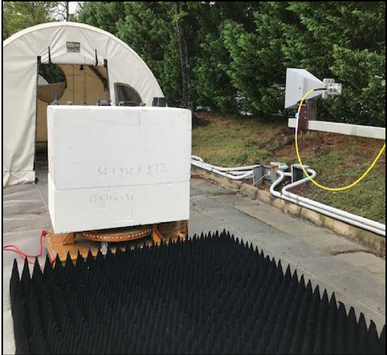
Photograph 1: Radiated Emissions Testing – Front View (Above 1 GHz)
