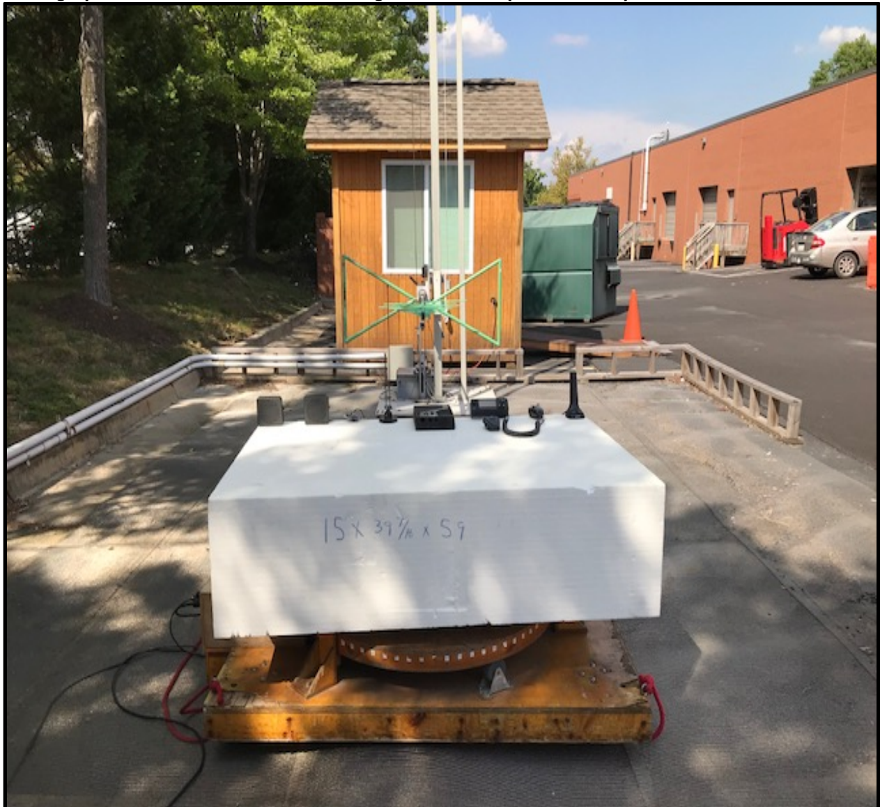
Photograph 3: Radiated Emissions Testing – Front View (Below 1 GHz)
