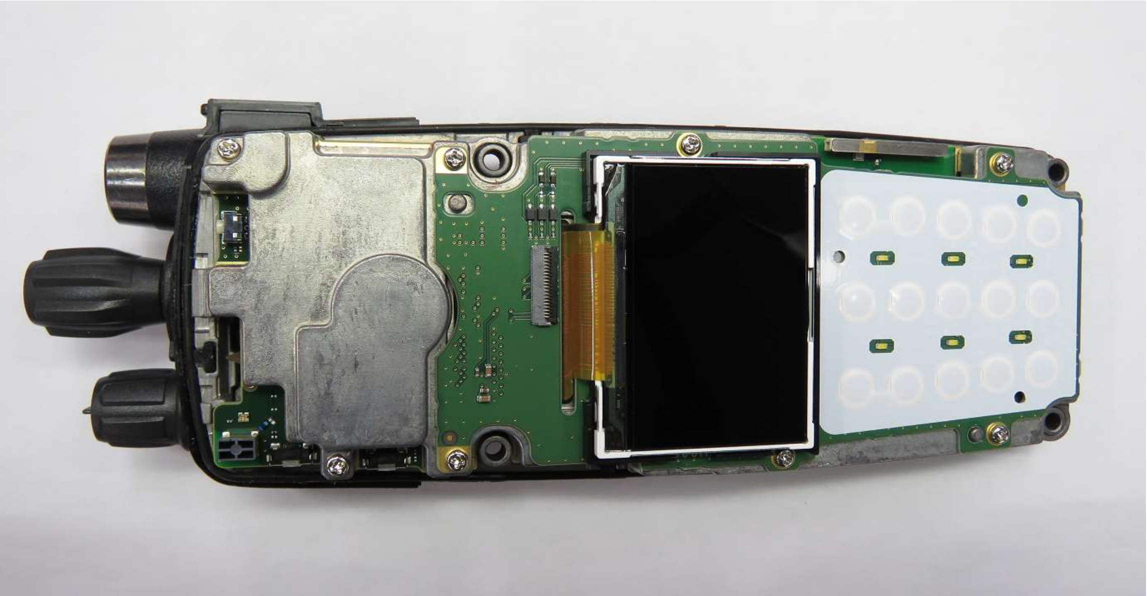
showing IF board and display when front cover is off
