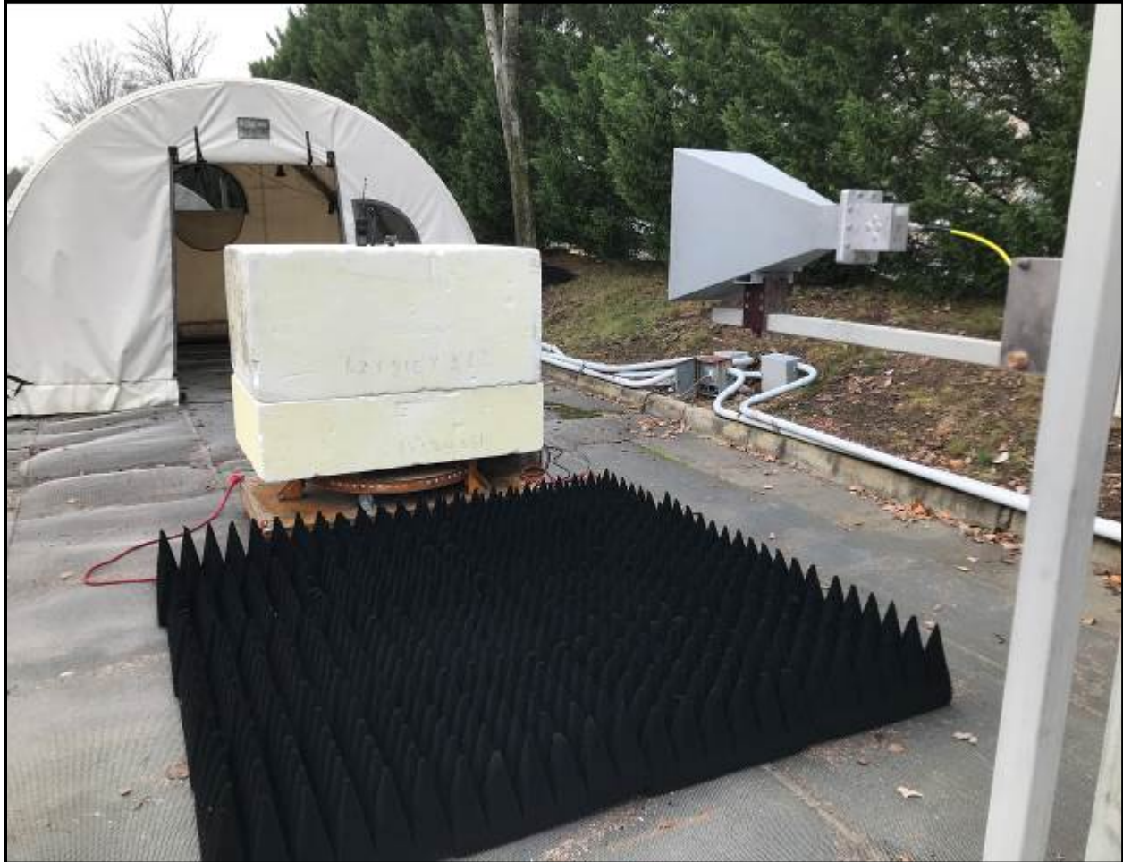
Photograph 1: Radiated Emissions Testing – Front View (Above 1 GHz)
