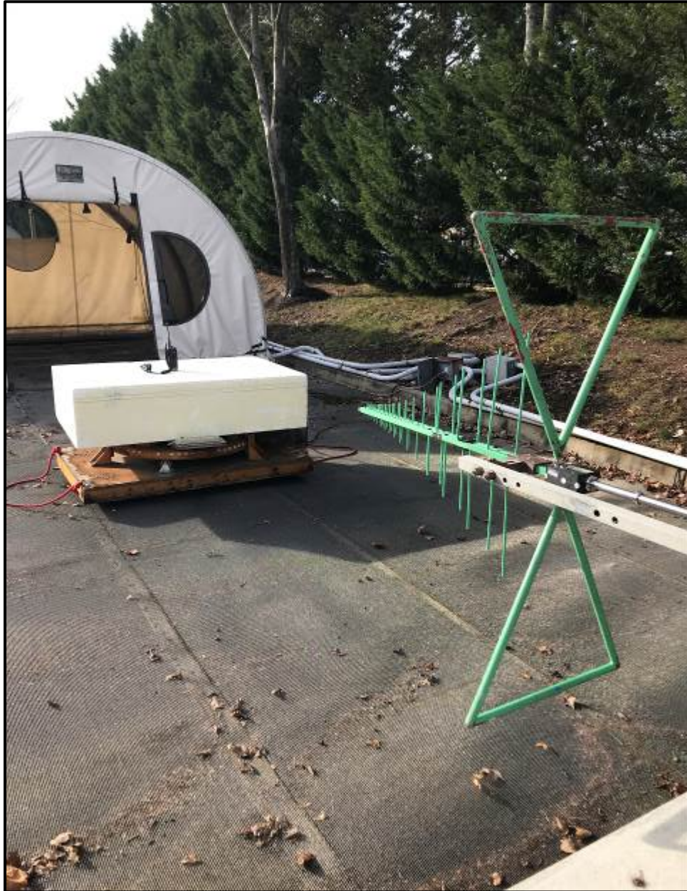
Photograph 3: Radiated Emissions Testing – Front View (Below 1 GHz)
