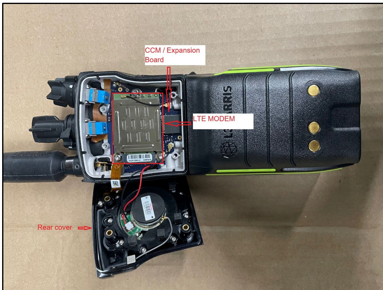
LTE Modem and CCM Board in XL-400P
