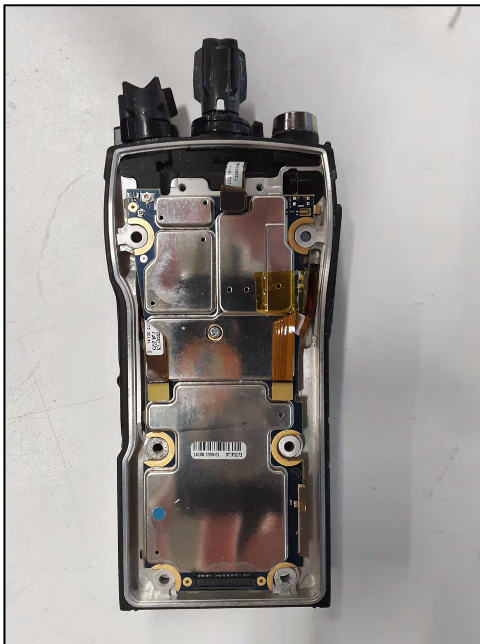
Main Board Installed in Chassis
